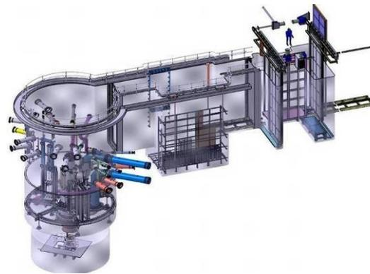
Fig. 5. Reactor pool and crossings.
