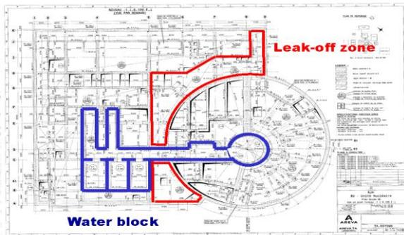
Fig. 4. Leak-off zone and water block.
