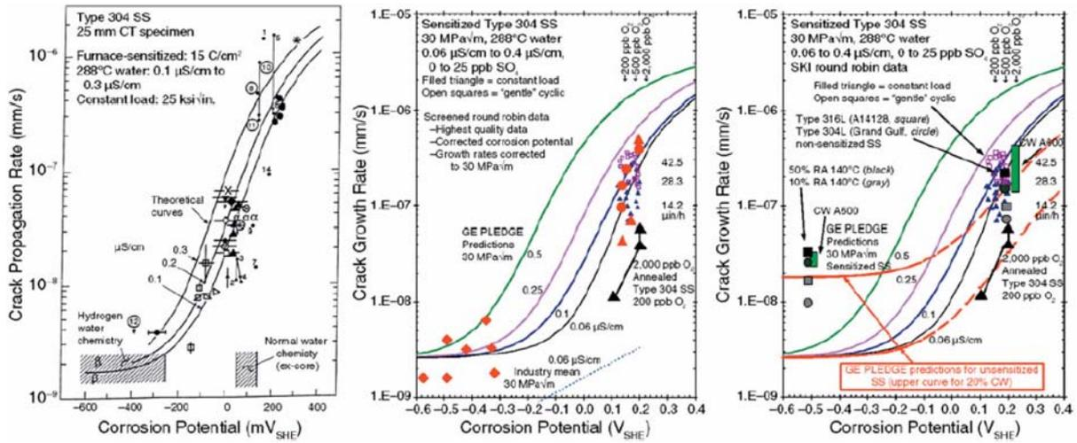
FIG. 6.6. Relationship between crack propagation rate and corrosion potential for sensitized Type 304 stainless steel in 288°C water under constant load and conductivity between 0.1 to 0.3  $\mu\text{S}/\text{cm}$ . The curves are the predicted relationships based on the slip-oxidation mechanism of crack propagation [6.14].
