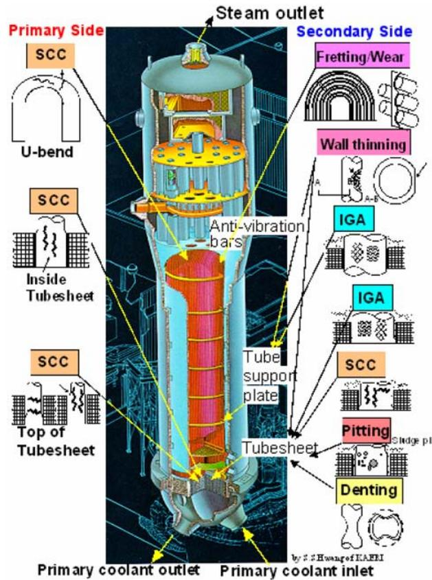
FIG. 3.11. Degradation mechanisms of various steam generator components.
