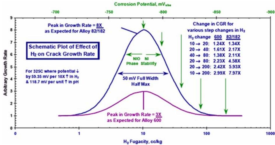
FIG. 6.22. Modelled crack growth rate for alloy 600 and alloy 182 for different hydrogen concentrations at 325°C.
