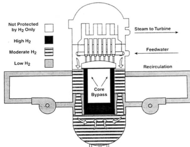
FIG. 6.7. Hydrogen water chemistry in reactor internals [6.15].
