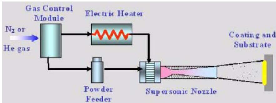
FIG. 6.12. Sketch of the cold spray corrosion resistant coating process.
