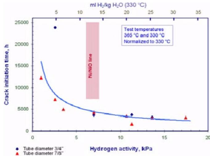
FIG. 2.10. The effect of hydrogen on initiation time. The data includes measurements at different temperatures normalized to the hydrogen partial pressure at 330°C [2.12].
