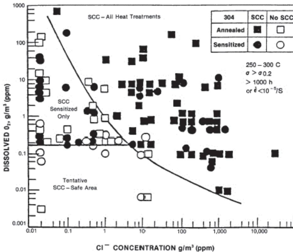
FIG. 2.19. Effect of chloride concentration on the critical concentration of dissolved oxygen for SCC in high temperature water [2.17].
