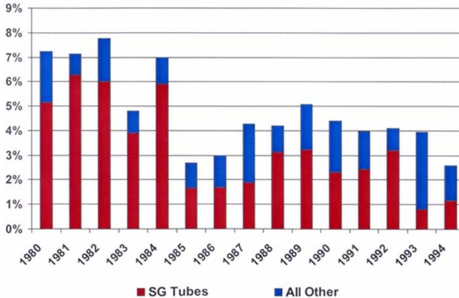
FIG. 3.5. Corrosion related capacity factor losses due to corrosion in PWRs [3.1].
