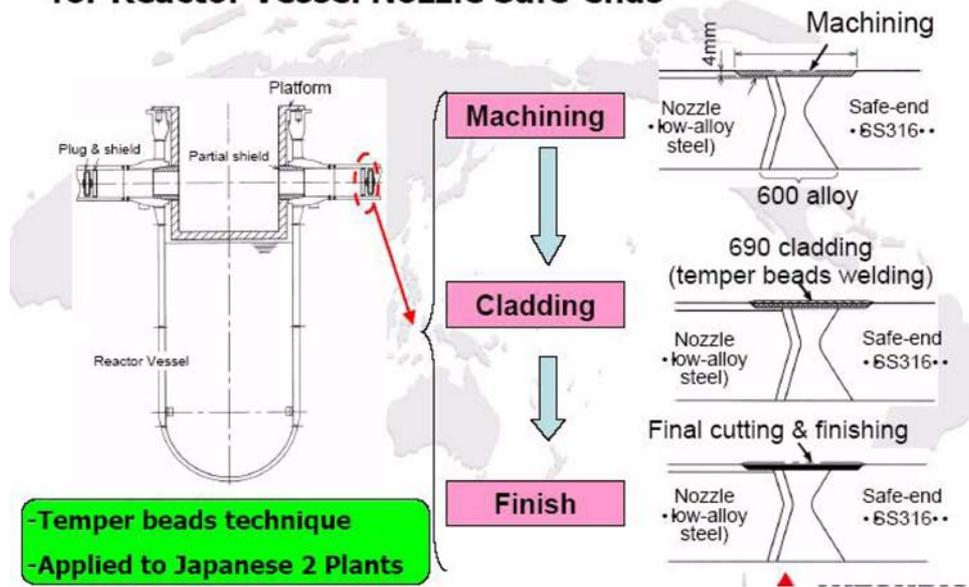
FIG. 6.14. 3-layer temper bead weld cladding technology.
