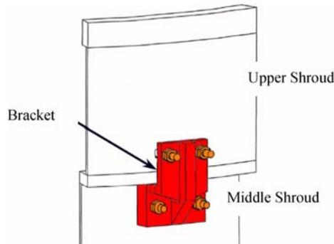
FIG. 6.11. Brackets repair technology.
