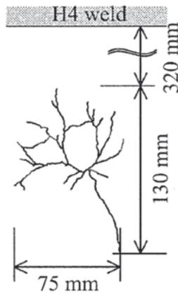
FIG. 3.4. An example of radial shaped SCC crack on a core shroud middle shell remote from any weld.
