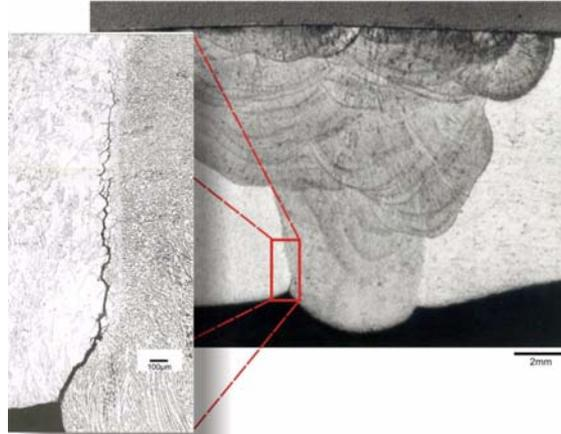
FIG. 3.2. IGSCC initiated at a notch root as a result of moderate cold work and a crevice condition.
