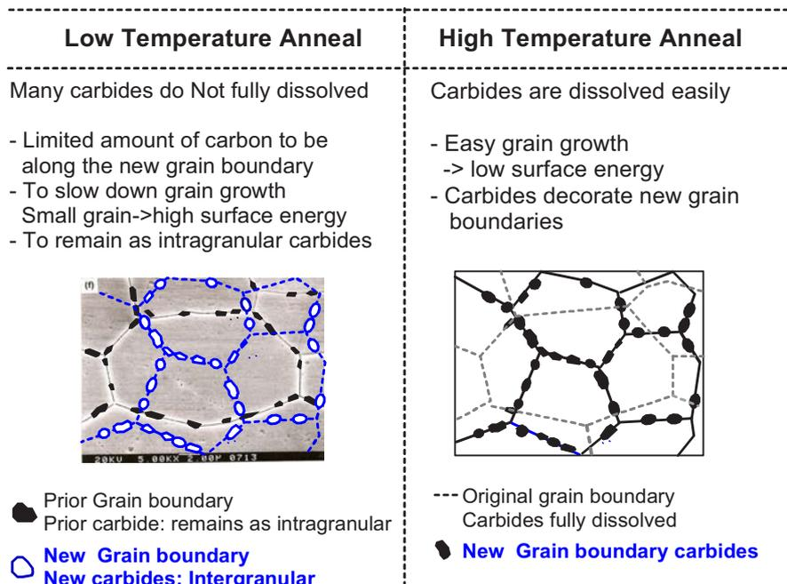
FIG. 2.5. Schematic of the carbide precipitation process.
