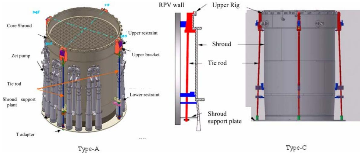
FIG. 6.10. Core shroud tie rods.
