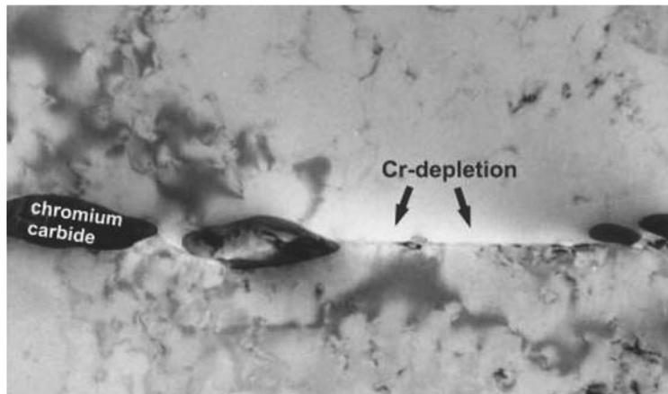
FIG. 2.3. Transmission electron microscope (TEM) image showing chromium carbide precipitates along a grain boundary and the zone of Cr-depletion [2.1].
