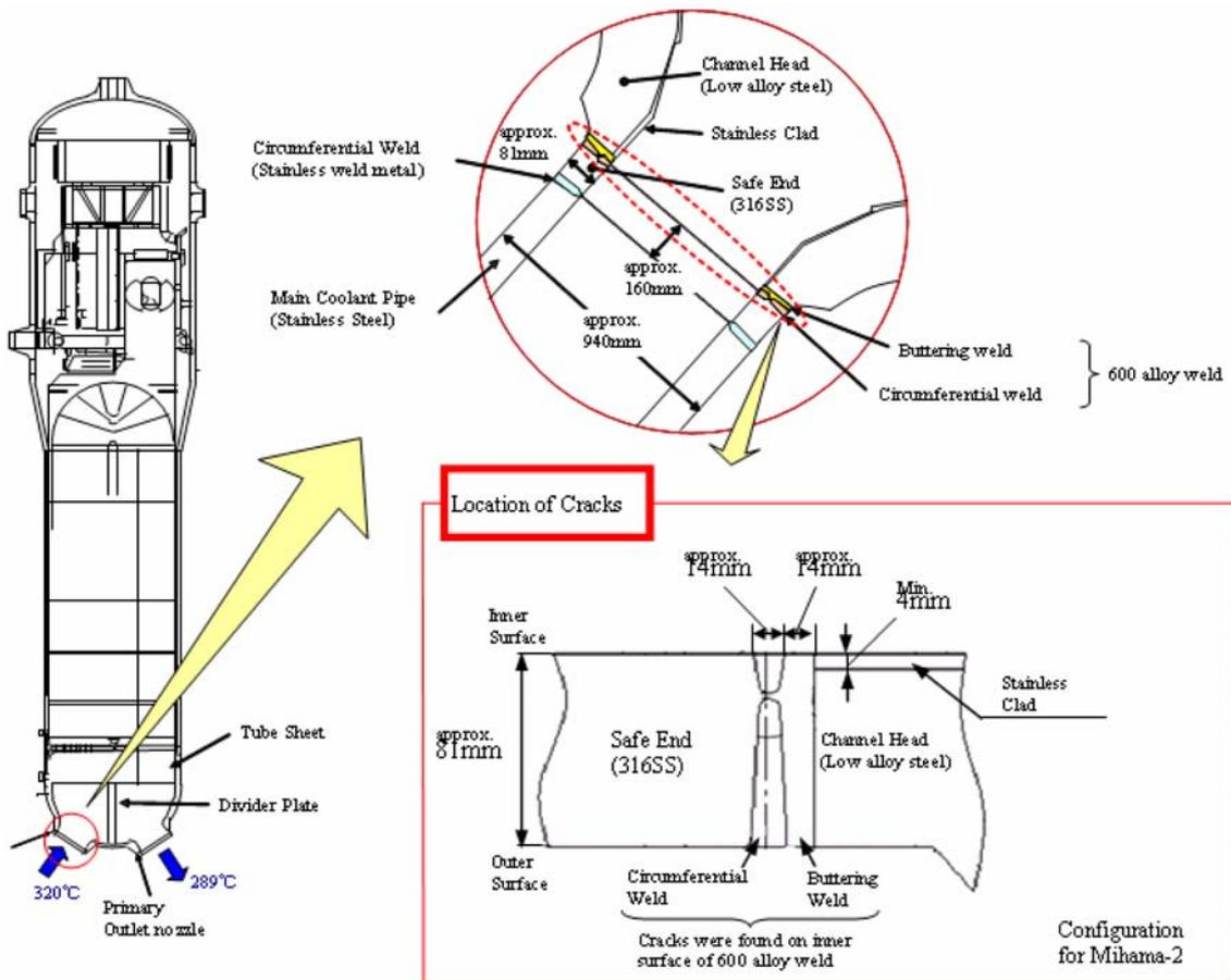
FIG. 3.12. Location of the primary inlet nozzles with indication.
