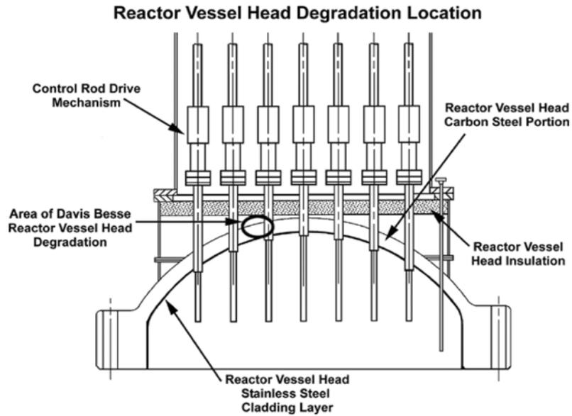
FIG. 3.6. PWR vessel head penetration cracking of alloy 600 allowed leakage of borated coolant to occur. This corroded the C&LAS RPV head externally down to the internal surface stainless steel cladding.
