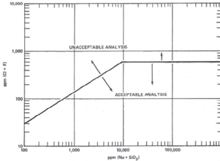
FIG. 2.18. Karnes ASME (USNRC Reg. Guide 1.36) showing the safe and unsafe areas for chloride and soluble silicate in insulation material.
