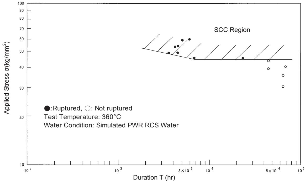
FIG. 2.12. Results of constant load PWSCC tests for alloy 600 base metal.
