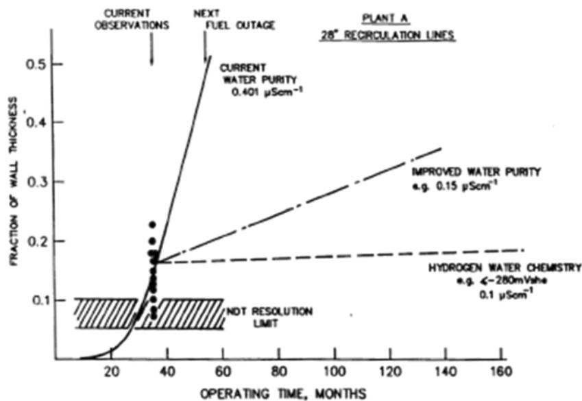
FIG. 6.9. Predicted response of defective piping for defined changes in water chemistry in BWR plant. The data points are the observed crack depth for type 304 stainless steel 28" recirculation piping in a given reactor.
