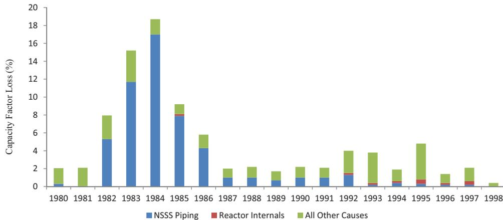
FIG. 3.1. Corrosion related capacity factor losses due to corrosion in BWRs [3.1].
