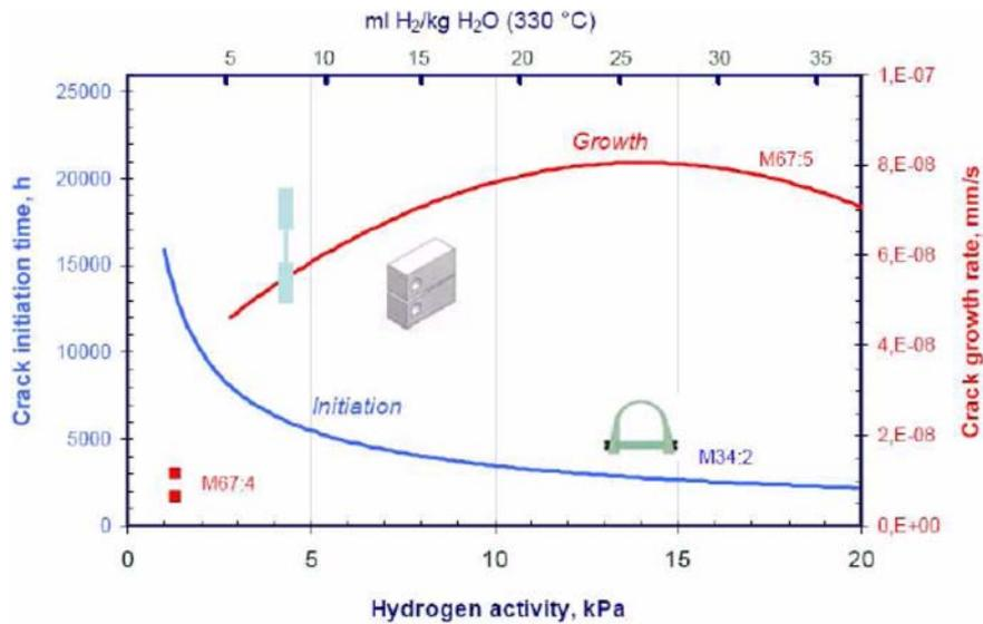
FIG. 2.11. Comparison of the effect of hydrogen on initiation and propagation of PWSCC in alloy 600 MA [2.12].
