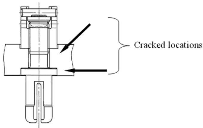
FIG. 3.13. Typical cracked location.
