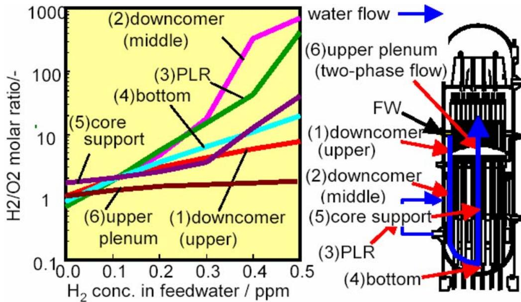
FIG. 6.8. ECP distribution for BWR internals.
