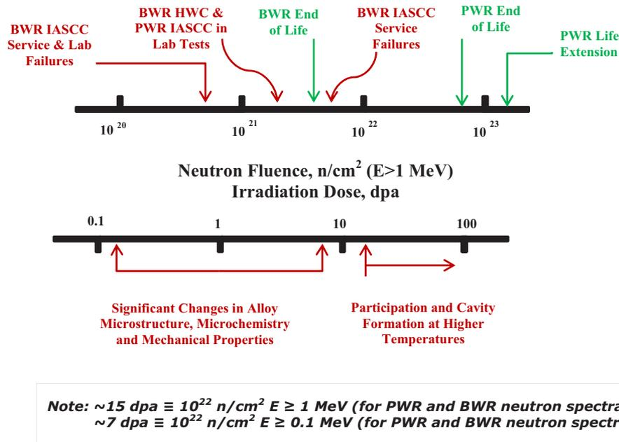
FIG. 2.7. Relationship between the irradiation effects and fluence.
