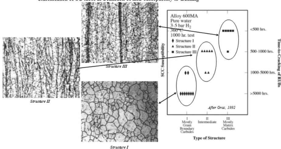
FIG. 2.6. Carbide classification system due to Vaillant.
