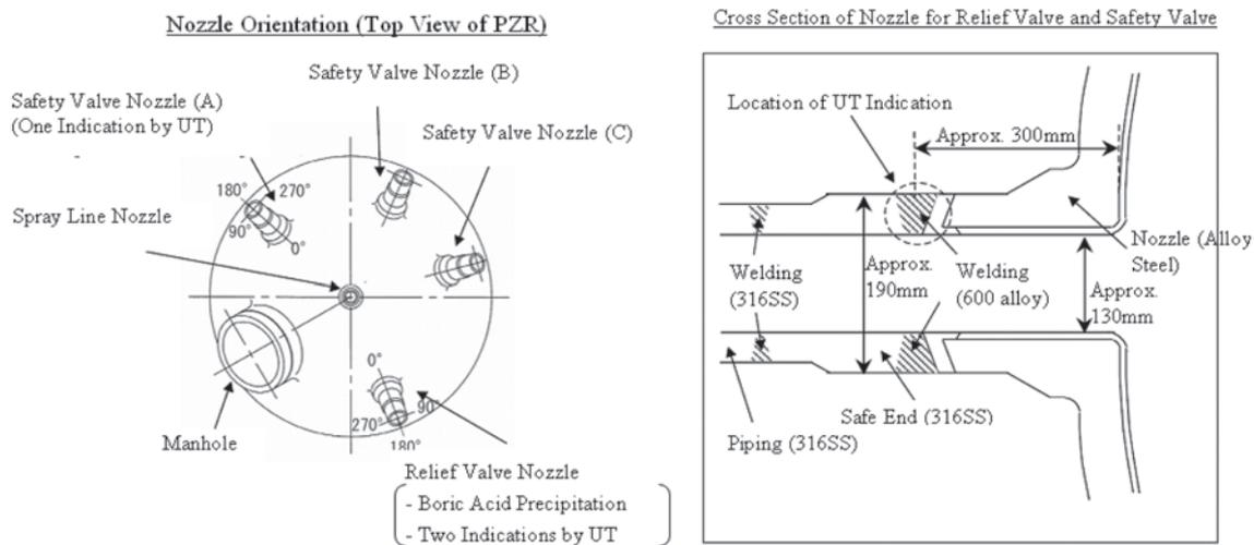
FIG. 3.10. Location of the nozzle with indication at Tsuruga Unit 2 [3.25].
