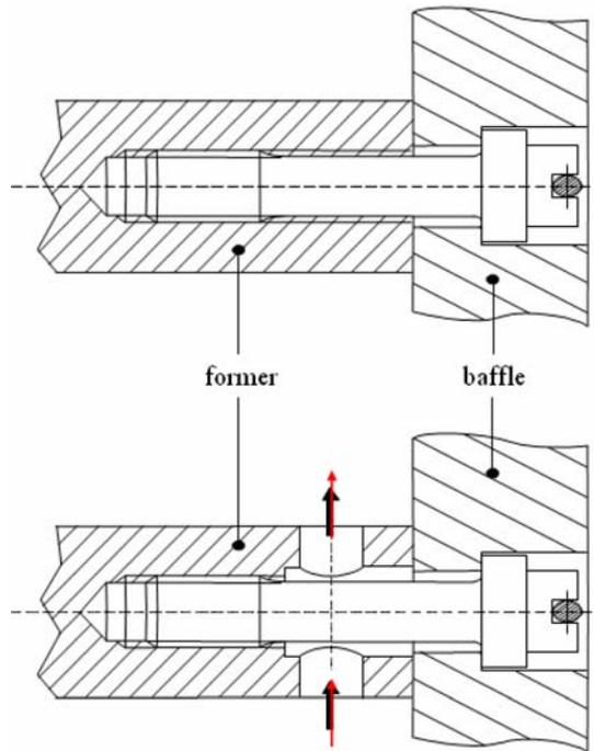
FIG. 6.15. Holes for water flow through formers to cool baffle bolts.
