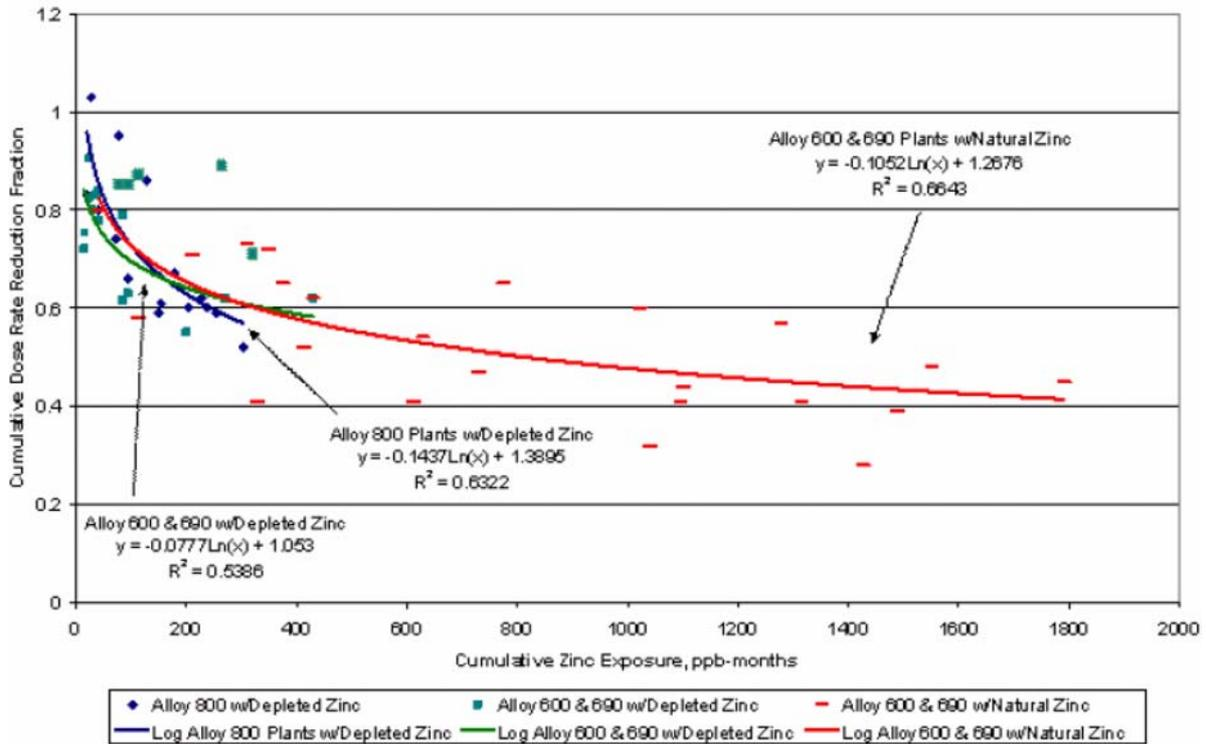
FIG. 6.21. Trends observed at US PWRs adding zinc, dose rate reduction vs. cumulative zinc exposure (ppb-mo). A significant fraction of the decrease in dose due to less corrosion product release is observed after ~300 ppb-mo of zinc exposure. Similar effects are anticipated for reduction in PWSCC [6.39].
