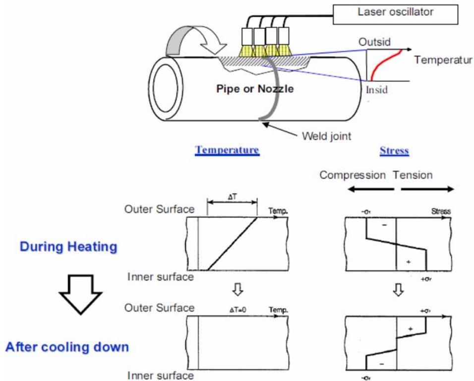
FIG. 6.20. Principle of L-SIP.
