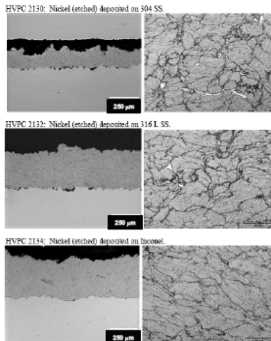
FIG. 6.13. Typical appearance of cold spray coatings in cross-section and on the surface. Both nickel and stainless steels coatings have been applied to type 304 SS, type 316 SS and alloy 600 substrates.
