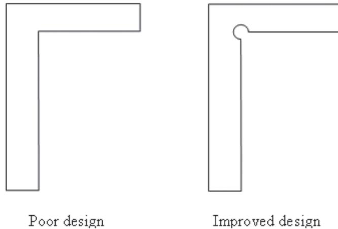
FIG. 6.3. Sketch of the tie rod upper support designs.
