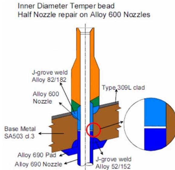
FIG. 6.25. Schematic of a crevice formed by the half nozzle repair.
