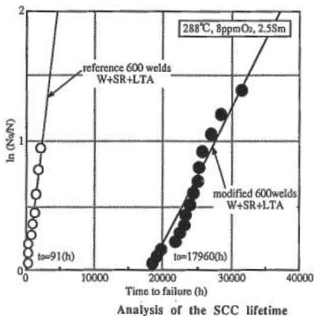
FIG. 6.1. SCC lifetime of conventional and modified Ni based alloys (alloy 600 welded with alloy 182) [6.7].
