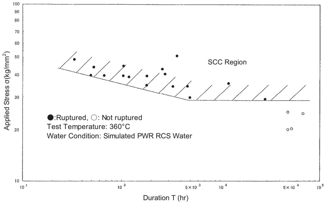
FIG. 2.13. Results of constant load PWSCC tests for alloy 132/82 weld metal.
