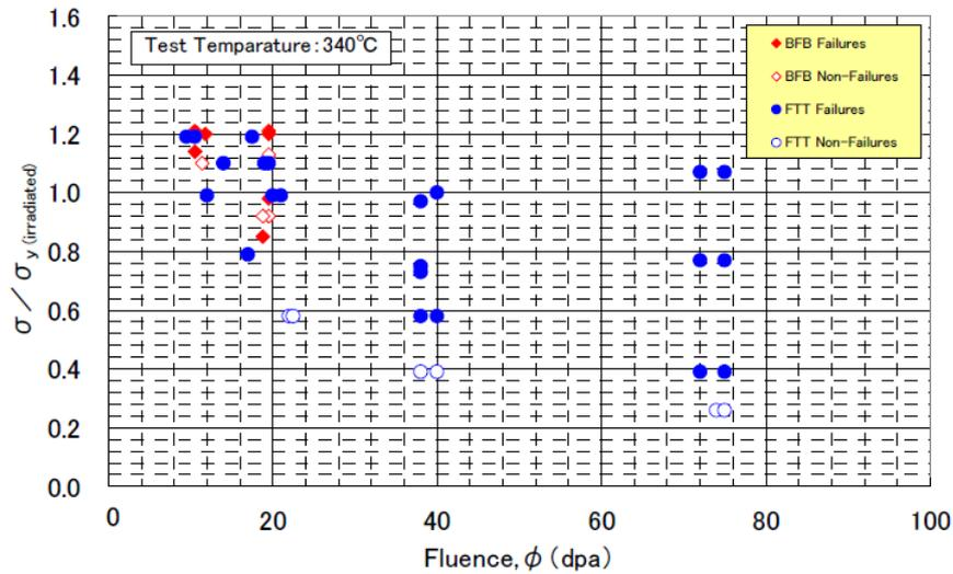
FIG. 2.16. SCC test results as stress/ $\sigma_y$  vs. fluence in dpa (at 340°C) [2.8].
