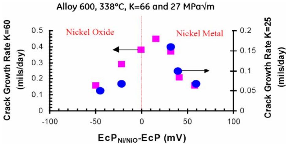
FIG. 2.8. Crack growth rate for alloy 600 in simulated PWR environment at 338°C [2.11].
