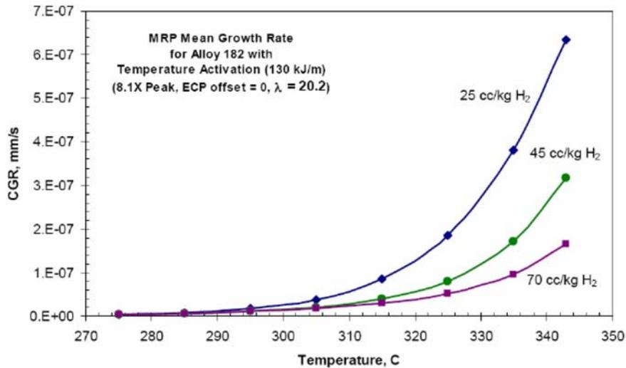
FIG. 2.9. Effect of temperature on PWSCC crack growth rate for alloy 182 [2.11].
