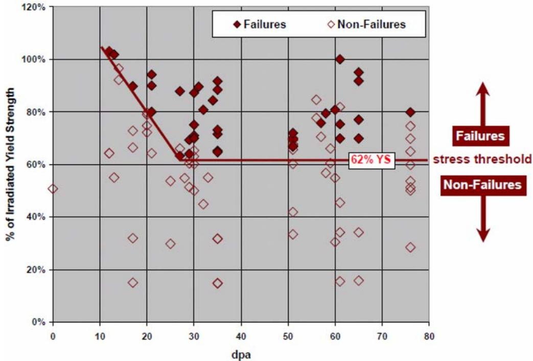
FIG. 2.17. SCC test results as stress/ $\sigma_y$  vs. fluence in dpa (at 340°C) [2.15].
