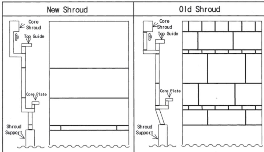
FIG. 6.2. Comparison between the old and new core shroud structures.
