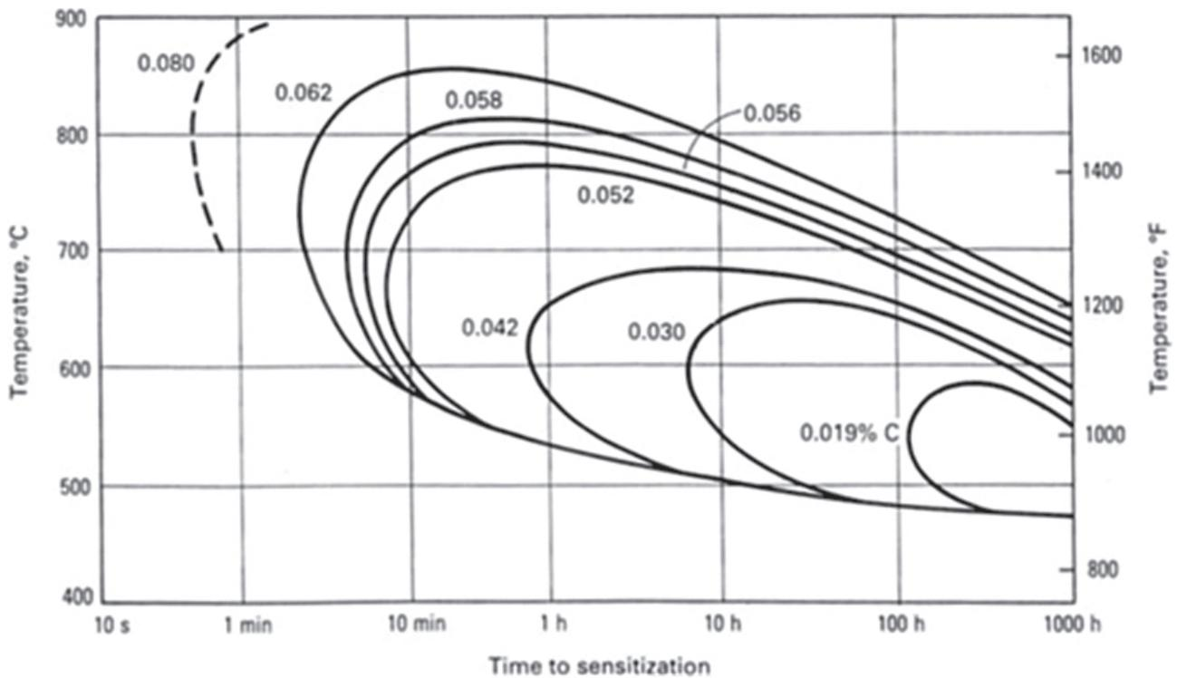
FIG. 2.2. Time-temperature-transformation (TTT) diagram for austenitic stainless steel showing the combinations of time, temperature and carbon content that lead to sensitization.
