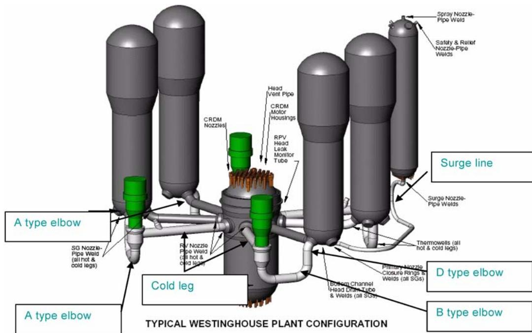
FIG. 7.1. Location of replaced RCL parts and elbows.
