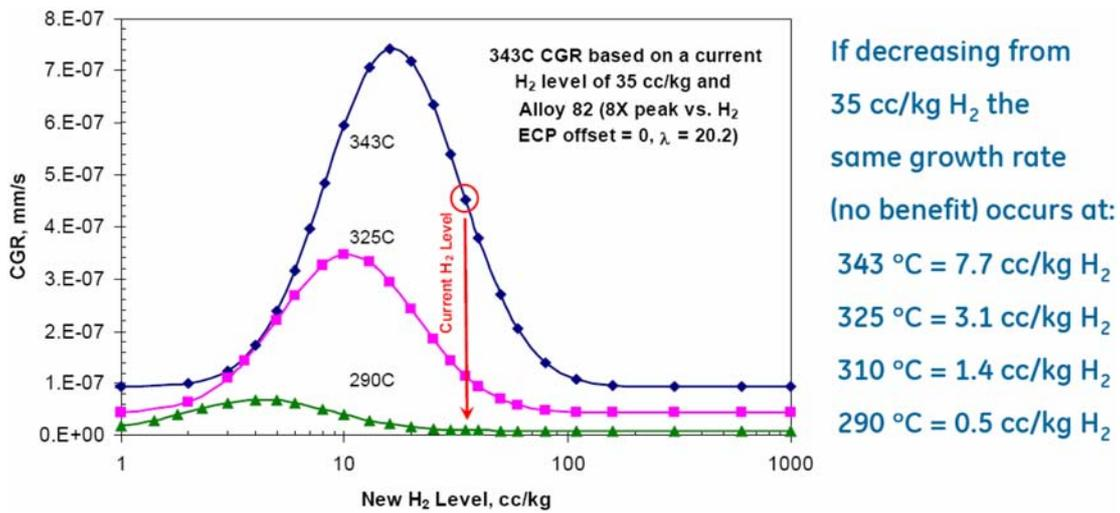
FIG. 6.23. Modelled crack growth rates for Inconel 82 showing the effect of hydrogen at different temperatures.
