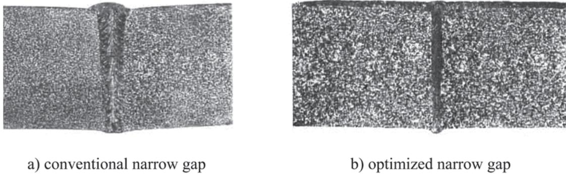
FIG. 6.4. Narrow gap welds in 30 mm austenitic stainless steel; the positive effect of the further reduced gap width on distortion can readily be seen.
