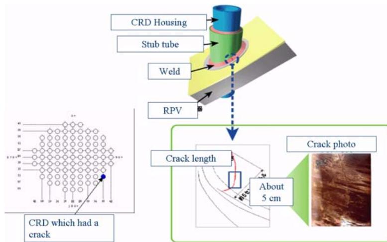
FIG. 3.3. CRD stub tube leak at Hamaoka NPP.
