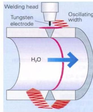
(b) Last pass heat sink welding (LPHSW)
