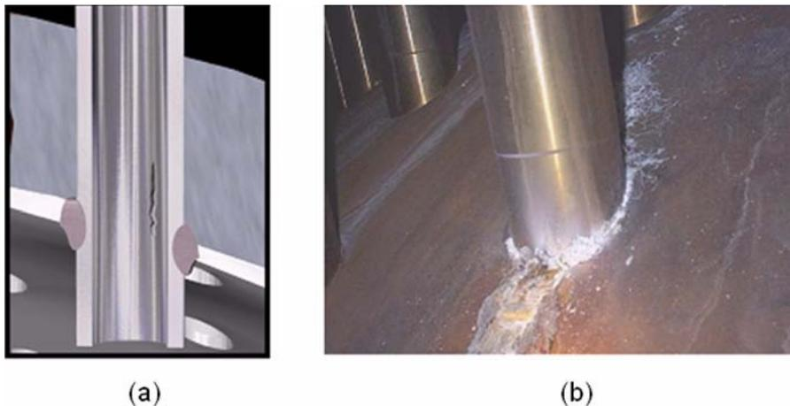
FIG. 3.7. (a) Depiction of a through-wall nozzle crack, (b) Typical appearance of 'popcorn' boron indications from leakage due to through-wall cracking.
