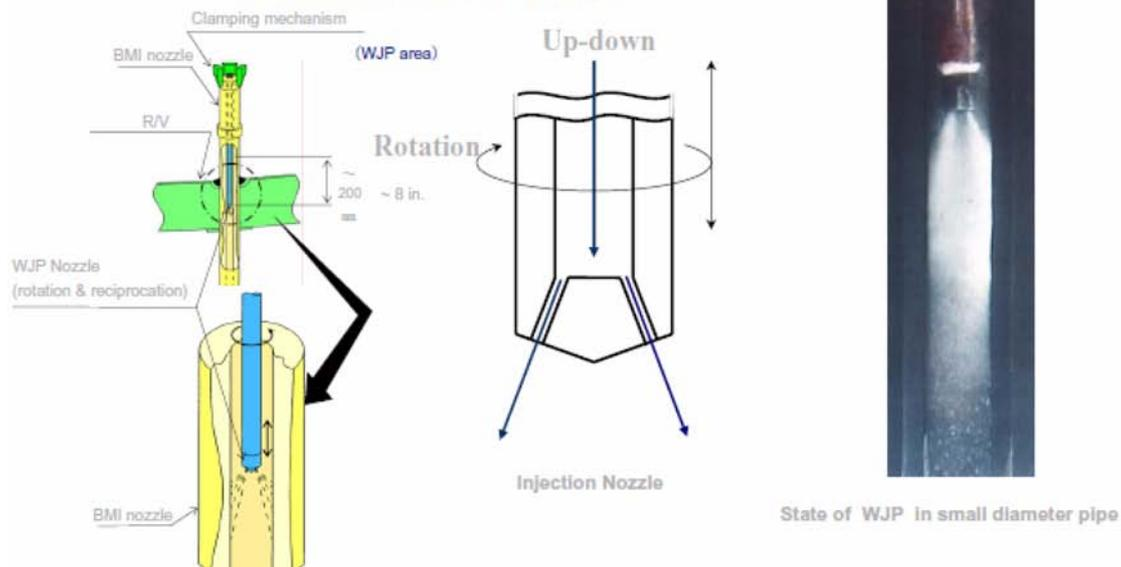
FIG. 6.19. Water jet peening process at the inner surface of a BMI nozzle.
