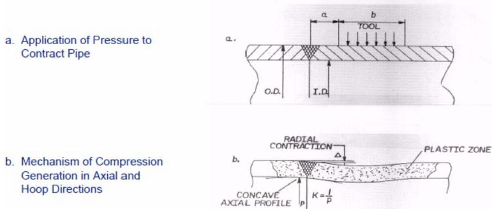
FIG. 6.17. Basic concept of MSIP: a clamp is applied on one side of a pipe weld to plastically deform the weld and in the process generates compressive stresses in both the axial and hoop directions.
