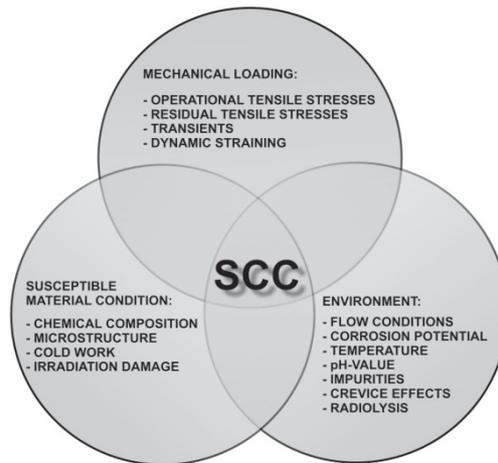
FIG. 2.1. Critical factors for stress corrosion cracking.
