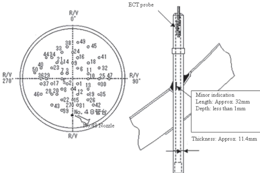
FIG. 3.9. Location of the BMI penetration nozzle Takahama Unit 1 with a small indication [3.24].
