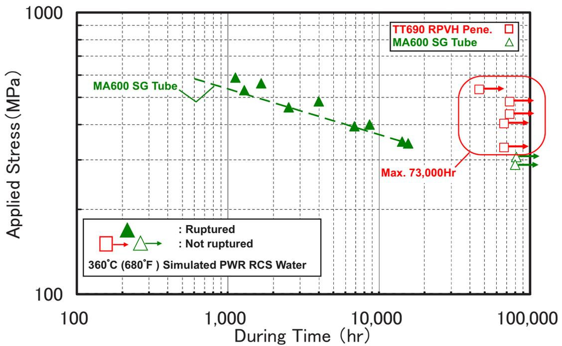
FIG. 2.14. Results of PWSCC tests on alloy 690 base metal and Alloy 600 base metal showing no cracking detected in alloy 690 after test times up to ~75 000 hours.
