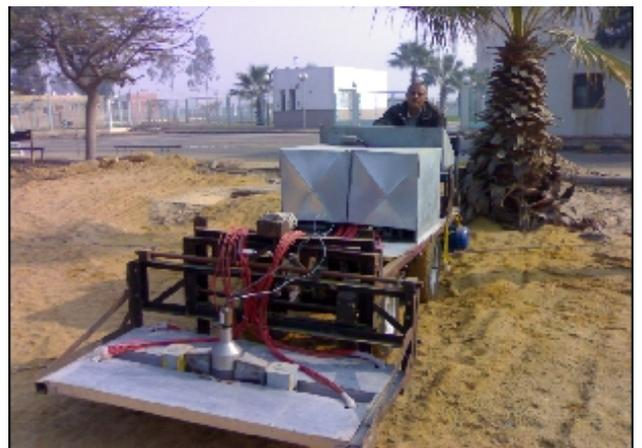
FIG. 1: Photograph of Egypt Scanning Landmine Detector, ESCALAD.
