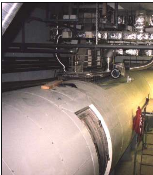
Ti foil between accelerator and reactor
