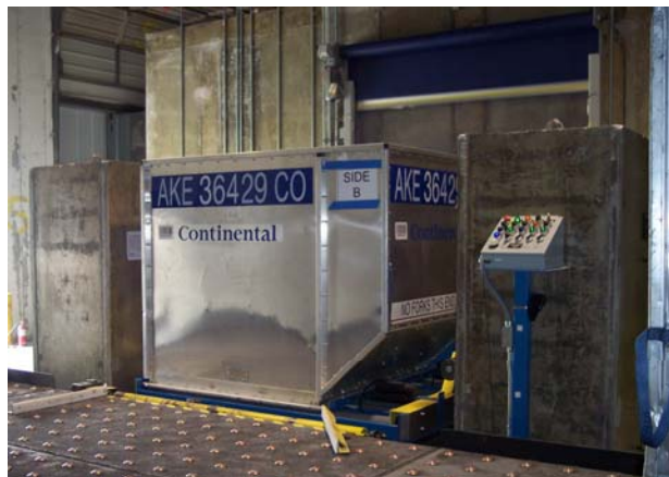
Rapiscan PFNA Air Cargo Inspection System
