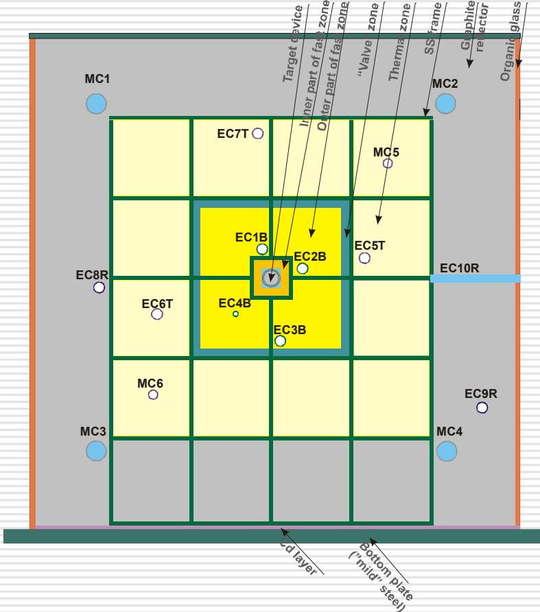
EC1B-EC4B – experimental channels in fast zone;
