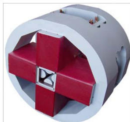
FIG. 6. Doublet of magnetic quadrupole lenses of new design.
