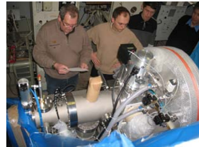
FIG. 8. Mass spectrometer units inspection after their transportation to IAP.
