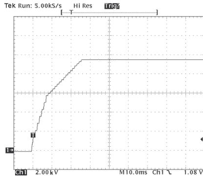
Fig. 10, Variable ramp start-up
