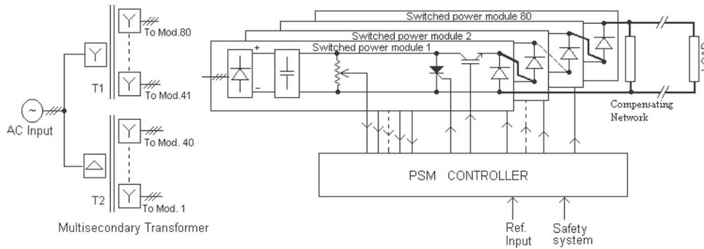
Fig. 3, Solid state high voltage power supply using PSM.
