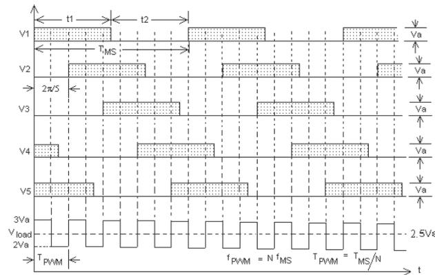
Fig. 2. Output Voltage with PSM and PWM for 5 SPMs.
