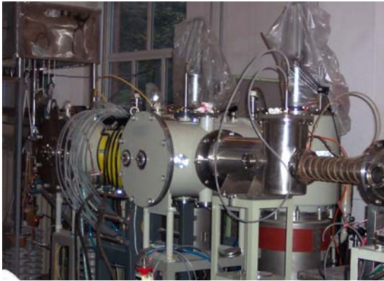
FIG. 3 The ADS ECR proton source.
