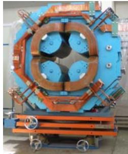
FIG. 11. The prototype RCS quadrupole magnet.
