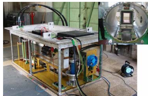
FIG. 14. The prototype extraction kicker (insert) and its pulse forming network for the CSNS RCS .
