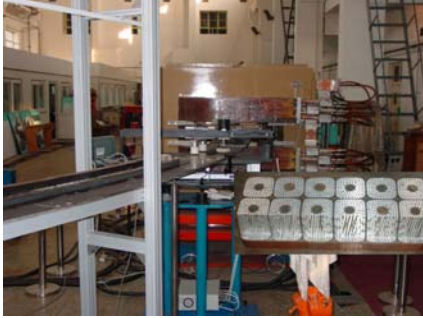
FIG. 9. The prototype RCS dipole magnet of stranded coil and the measurement system.
