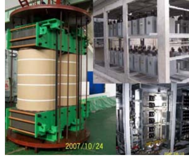
FIG. 10 The prototype power supply for the dipole magnet (choke, capacitor bank, and supply).
