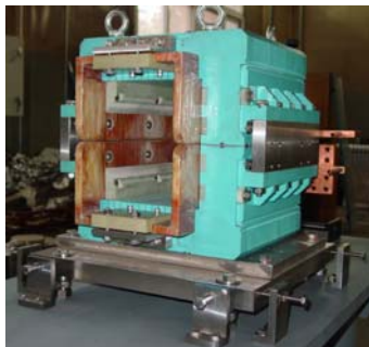
FIG. 13. The prototype injection magnet for the CSNS RCS.
