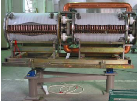
Fig. 15 The prototype ferrite-loaded RF cavity for the CSNS RCS
