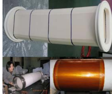
FIG. 12. The short prototype of the dipole ceramic chamber (upper) and two full-size quadrupole ceramic chambers (lower) .
