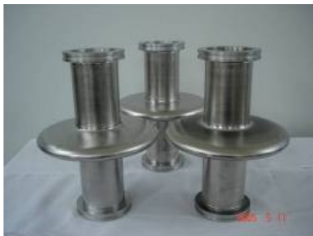
FIG. 8 \beta=0.45 SC cavities at 1.3 GHz with the measured Q_0 > 1 \times 10^9 .
