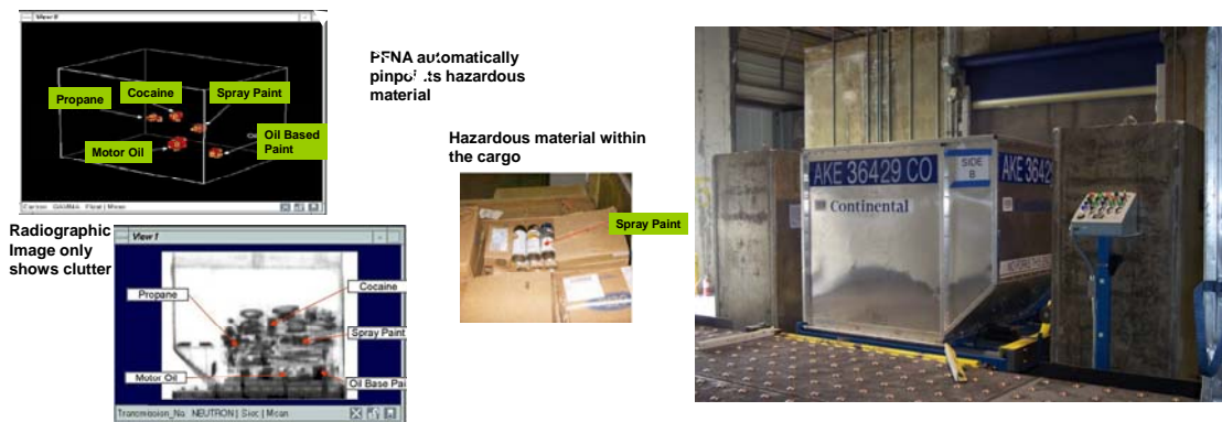
FIG. 12. Detection of small hazardous substances (left) in air cargo container by the PFNA technique. PFNA Houston air cargo prototype system (on right) [ see also this proceedings].
