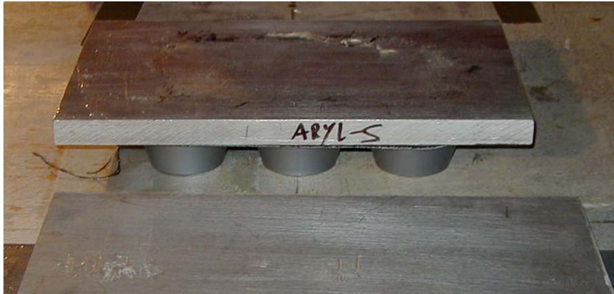
FIG 2. Carbon-fiber composite cups X-ray cured in a thin steel mold beneath a 2 centimeter thick aluminum plate to simulate a thick walled metal mold.
