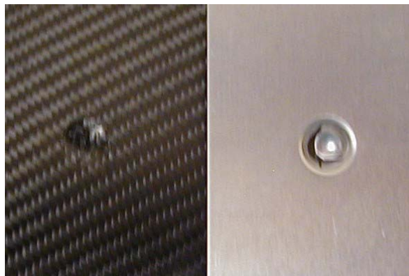
FIG. 1. Tup impacted at the same force: a four-ply X-ray cured carbon-fiber composite panel and aluminum plate of the same thickness. Carbon-fiber was indented; aluminum plate was fractured.
