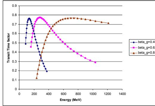
FIG. 4. Transit time factor curves for 3 constant beta cavities.
