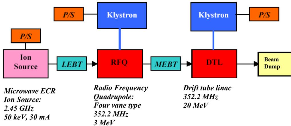
FIG. 1. Configuration of the 20 MeV linac for LEHIPA.
