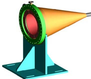
FIG. 3. Beam dump for the 20 MeV LEHIPA.
