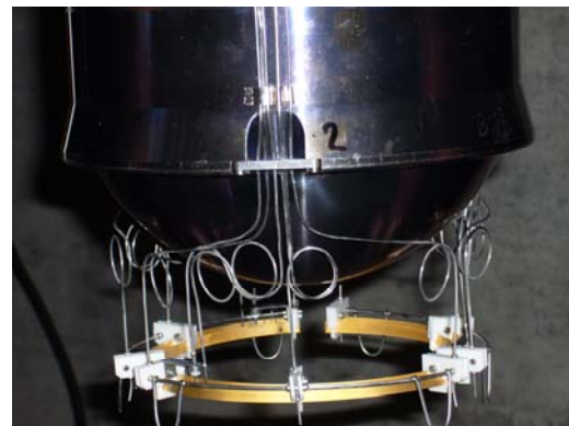
Figure 6: MEGAPIE leak detector mounted at the beam entrance calotte of the liquid metal container
