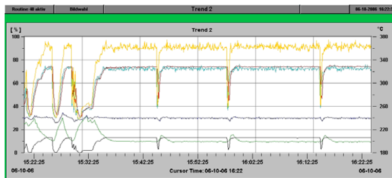
Figure 2: Time history of relevant temperatures responding to beam trips from full power
