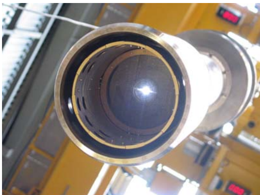
Figure 5: VIMOS head with a Tungsten wire mesh to be installed close in front of the target entrance window
