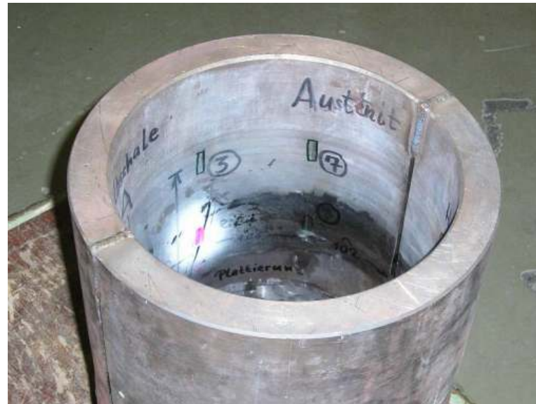
FIG. 4. Bi-metallic test specimen (OD 332 mm / 32 mm wall thickness)
