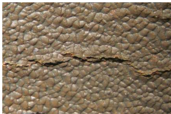
FIG. 2. Inside Surface of Degraded Feeder
