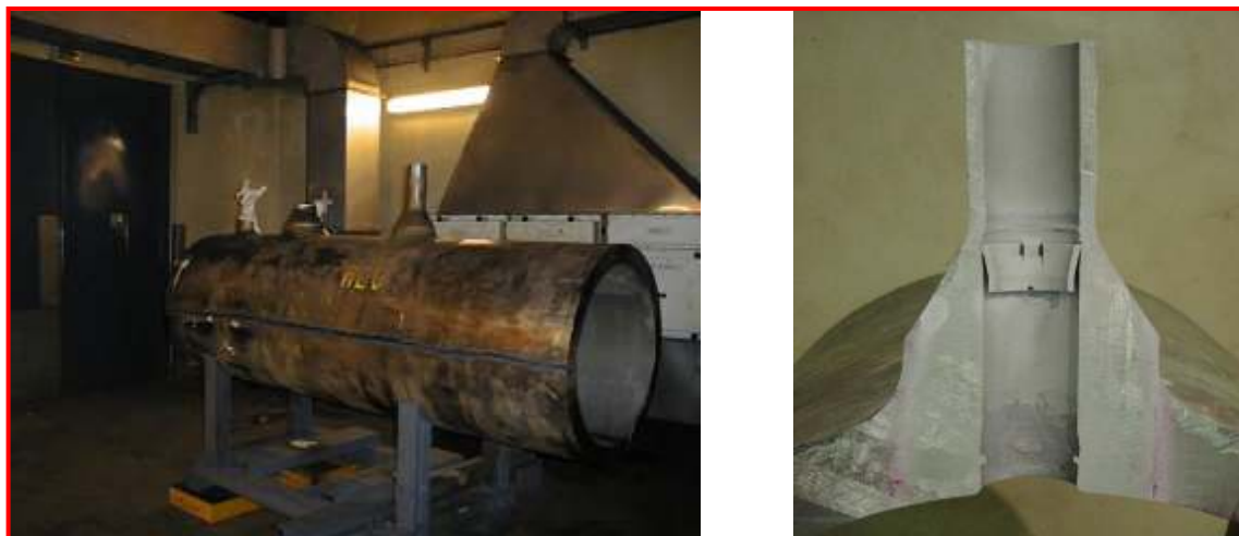
FIG. 14 Destructive examination of Fessenheim 1 CVCS nozzle
