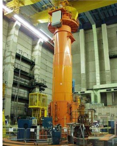
*Transfer flask for large primary components in position on reactor top*
