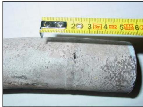
*Phenix – Nitriding defect on the steam tube of steam generator – Sodium/water reaction n°5*
