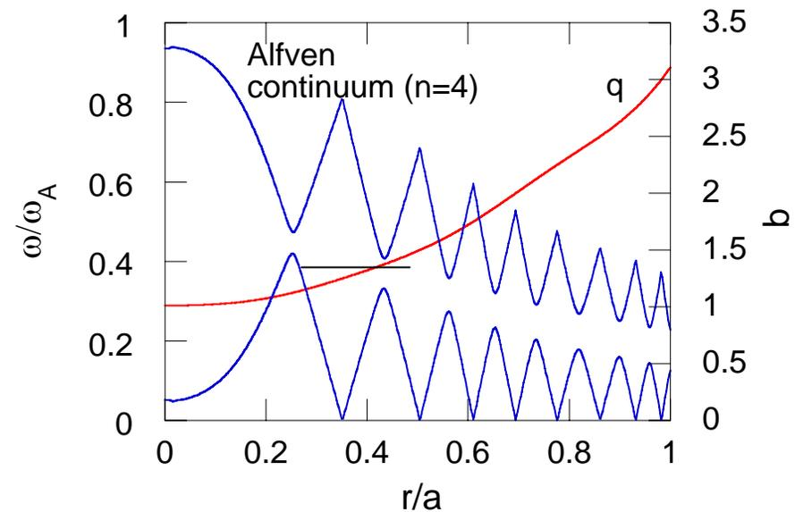
Alfvén continuous spectra with  $n=4$ , safety factor profile, and frequency and location of the most unstable  $n=4$  TAE.
