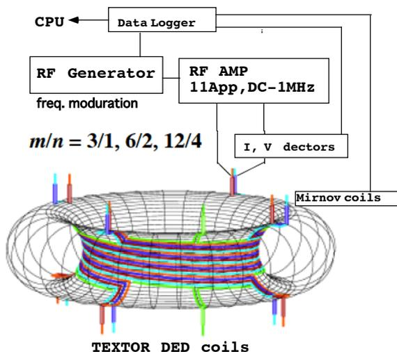
Fig. 1 DED coils and AEs antenna system
