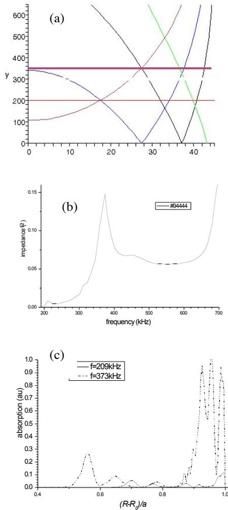
Fig.6 (a) Alfvén wave continuum frequency for  $n= -1$ ,  $m=1,2,3,4$ , (b) coil impedance spectrum and (c) power absorption profile.  $n_{e0}=3.2 \times 10^{19} \text{m}^{-3}$ ,  $B_t=2.25\text{T}$ ,  $D_2$   $q_0=1.25$ ,  $I_p=300\text{kA}$
