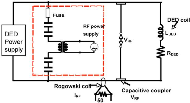
Fig. 2 Rf antenna circuit and impedance diagnostics
