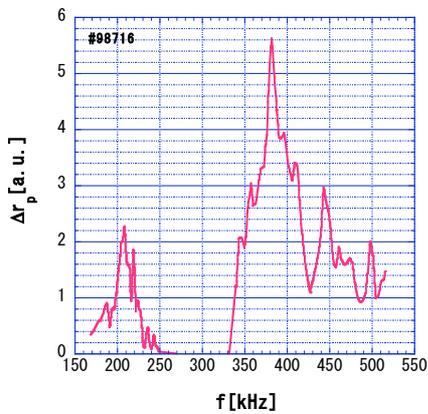
Fig. 5 Power spectrum of the change in the coil loading resistance from the vacuum.  $Bt=2.25\text{T}$ ,  $\langle n_e \rangle = 3.2 \times 10^{19} \text{m}^{-3}$ ,  $I_{DED}=1.5\text{kA}$ ,  $+1\text{kHz}$ .
