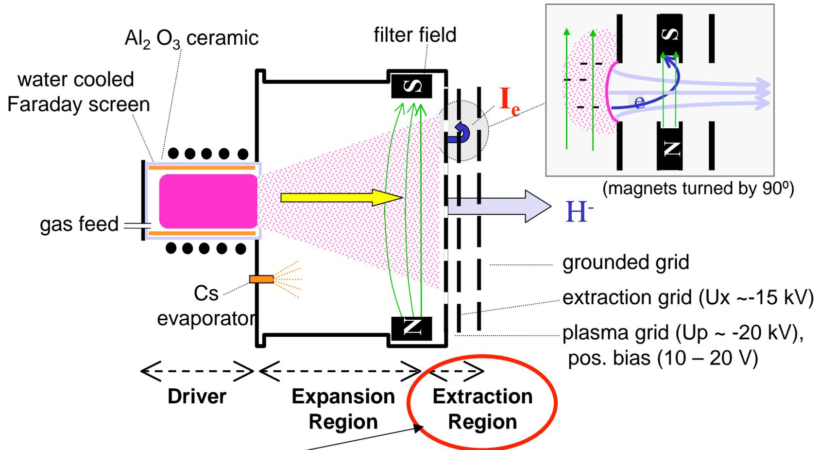
**critical: power to extr. grid =  $I_e \times (U_p - U_x)$**
