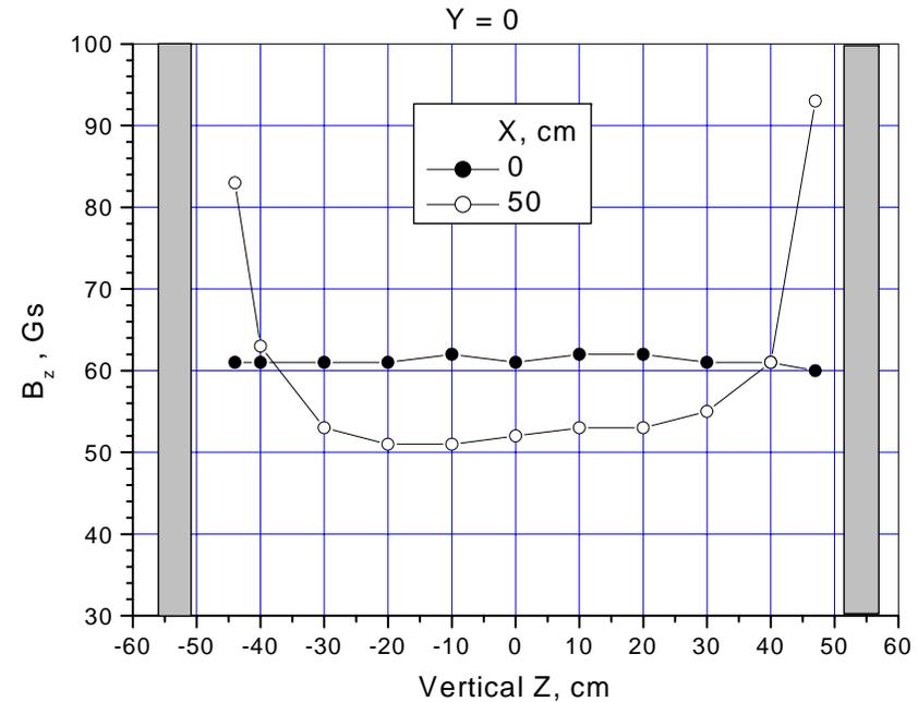
Advantage of such MS configuration - **very uniform  $B_z$**  inside the “magnetic box”.
