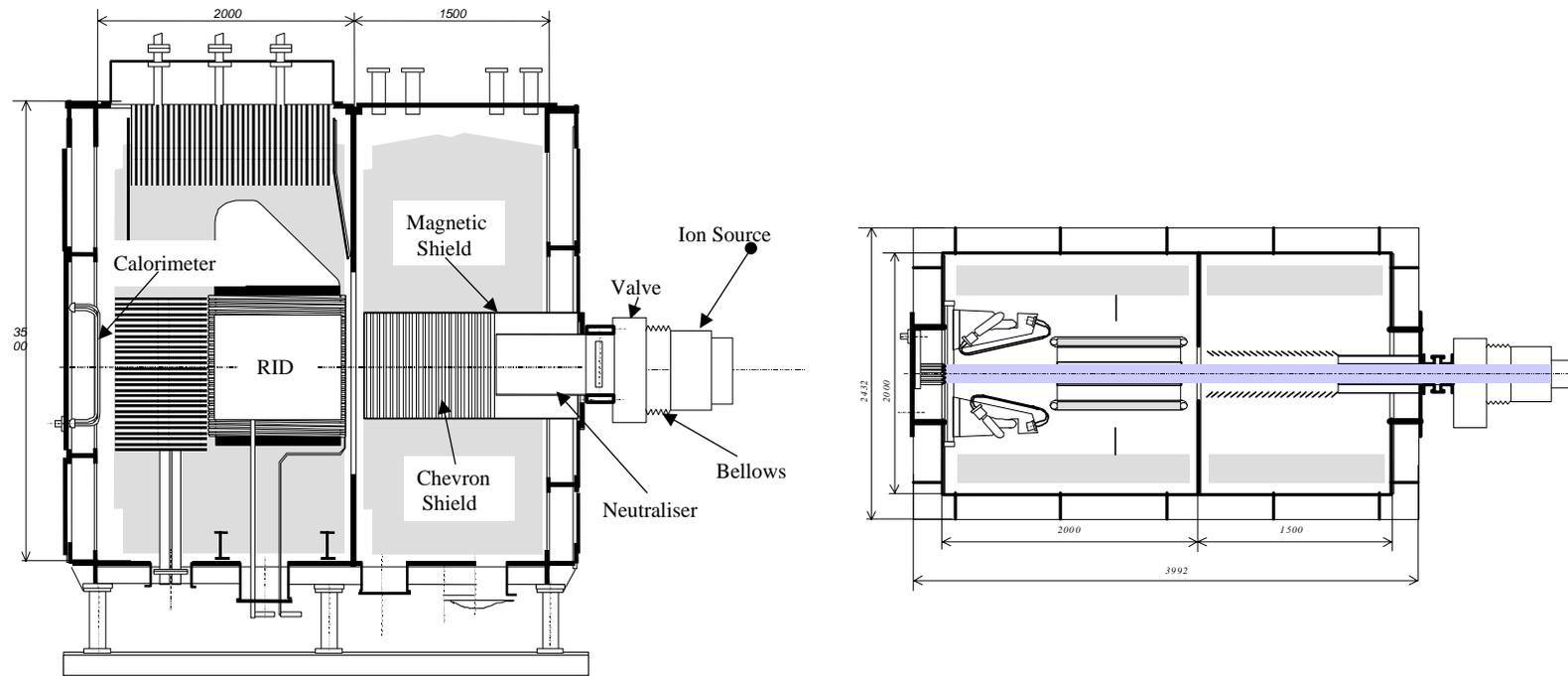
The experimental RID layout in vacuum vessel
