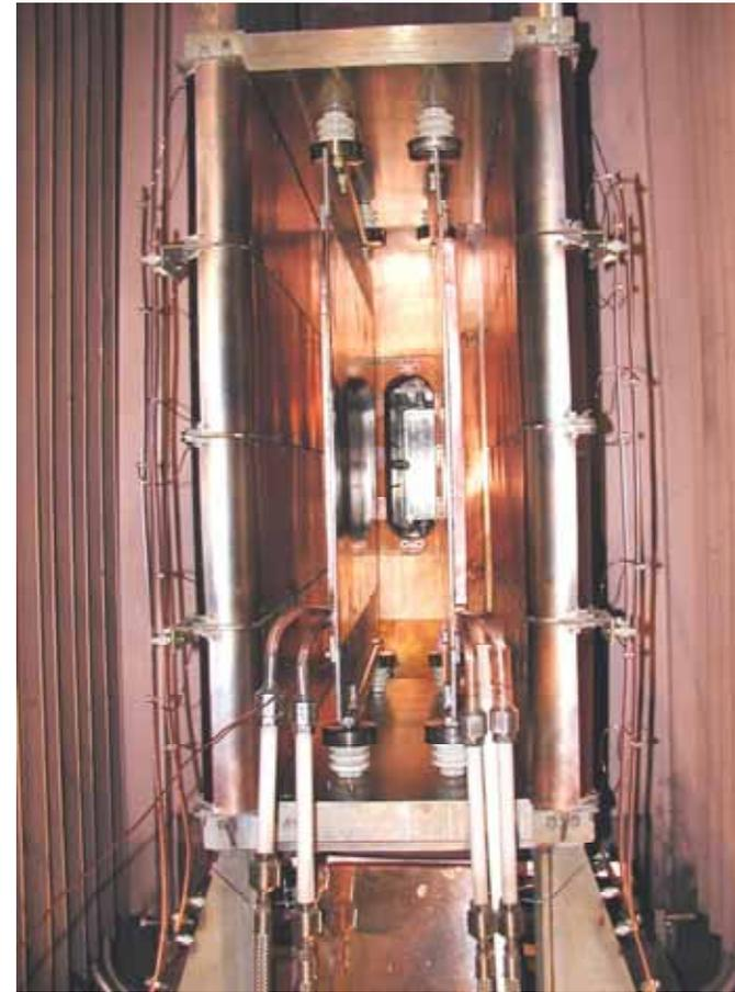
Views of the RID magnetic system and the RID inside the IREK vacuum vessel (deflecting panel is on the right).
