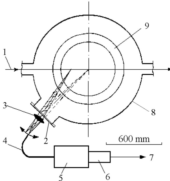
*1 –laser ray; 2 –quartz window; 3 –scanning system lens; 4 –light guide;*
