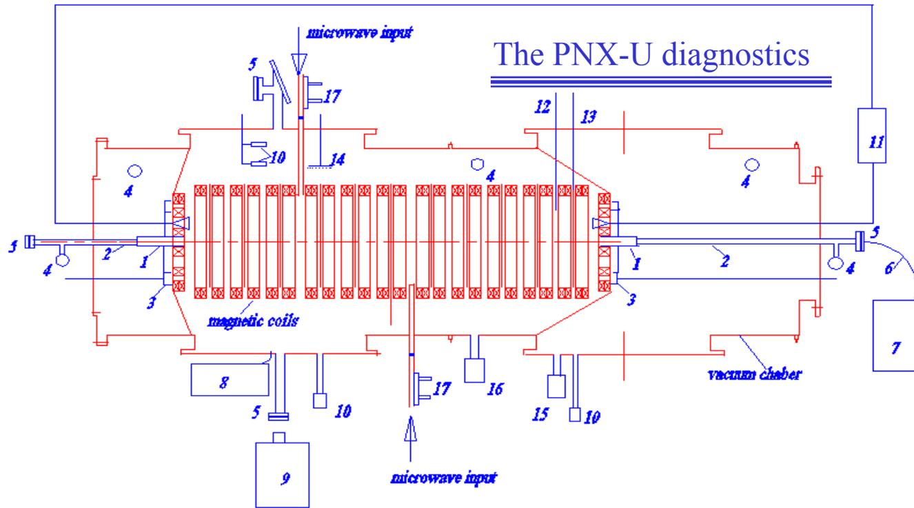
1-axial plasma collector, 2- tube, 3- end slit plasma collector, 4-gauge, 5-optical window, 6- optical conductor, 7- optical plasma radiation monochromator, 8- laser fluorescence monochromator, 9- excimer laser, 10- multygrid plasma flow analyser, 11- 4-mm interferometer, 12- movable Langmuir probe in gap, 13- movable Langmuir probe in slit, 14- Langmuir probe system placed outside coils, 15- photomultiplier, 16- gas mass spectrometer, 17- microwave directional coupler.
