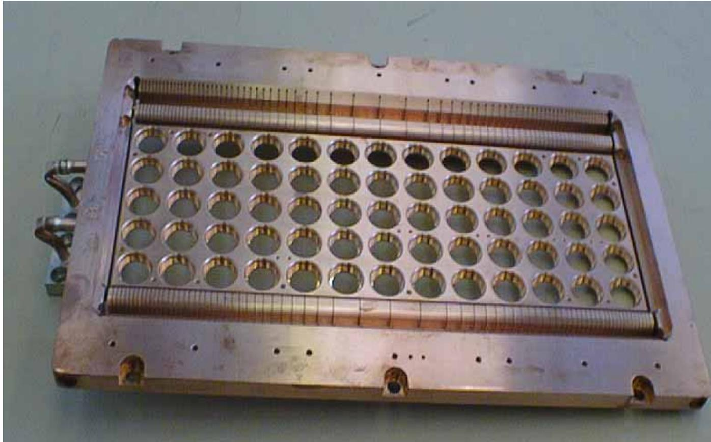
**Cu/Cr/Zr long pulse grid (6 mm thick).**
