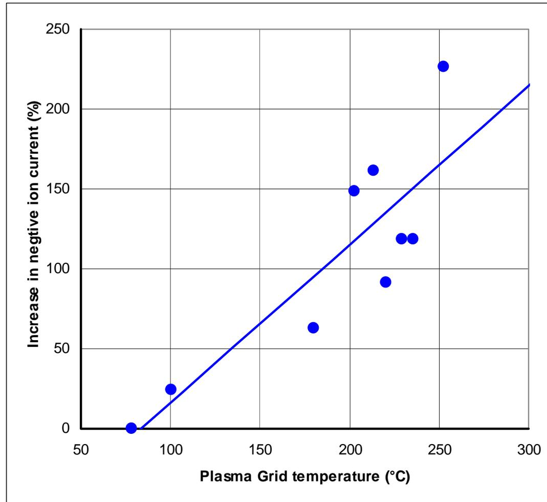
**Effect of plasma grid temperature on the accelerated negative ion current with the KAMABOKO III ion source.**
