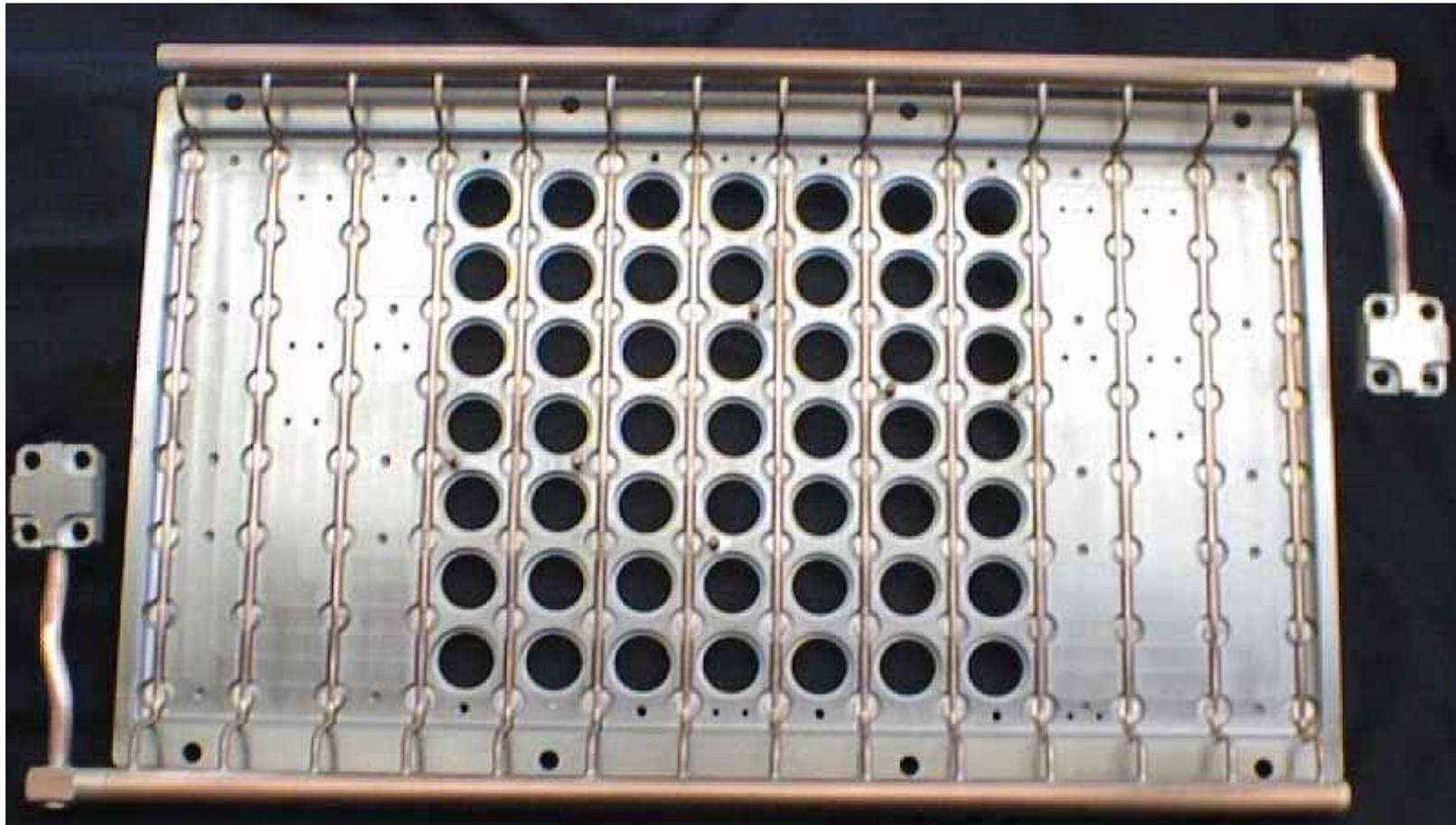
**Molybdenum long pulse grid (6 mm thick).**
