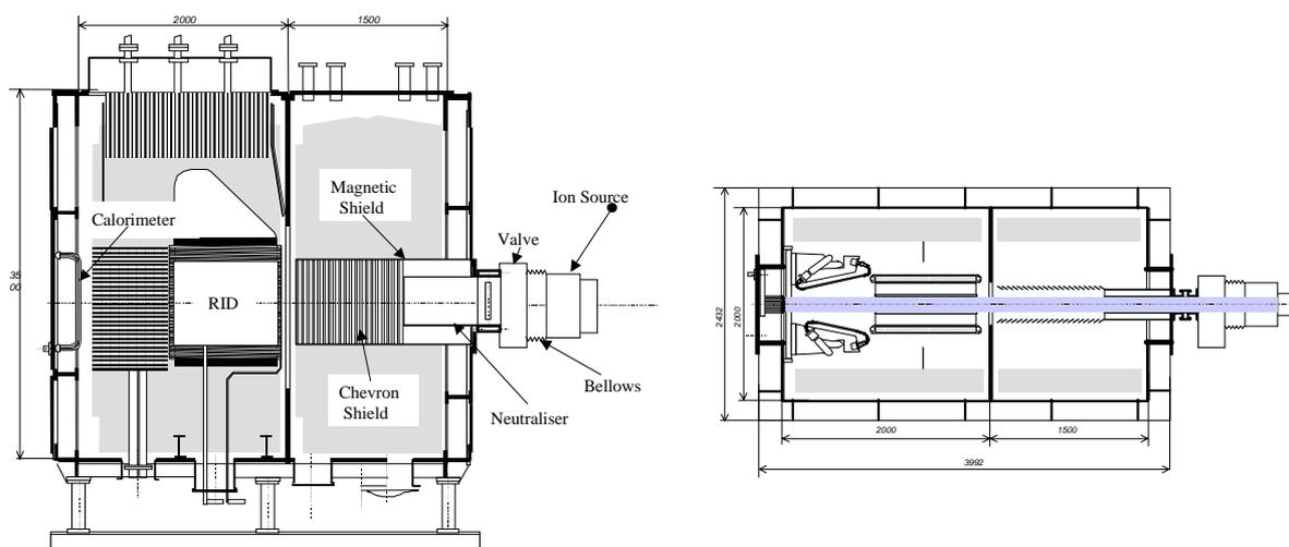
Fig.1. Layout of the electrostatic RID in the IREK test injector vacuum vessel
