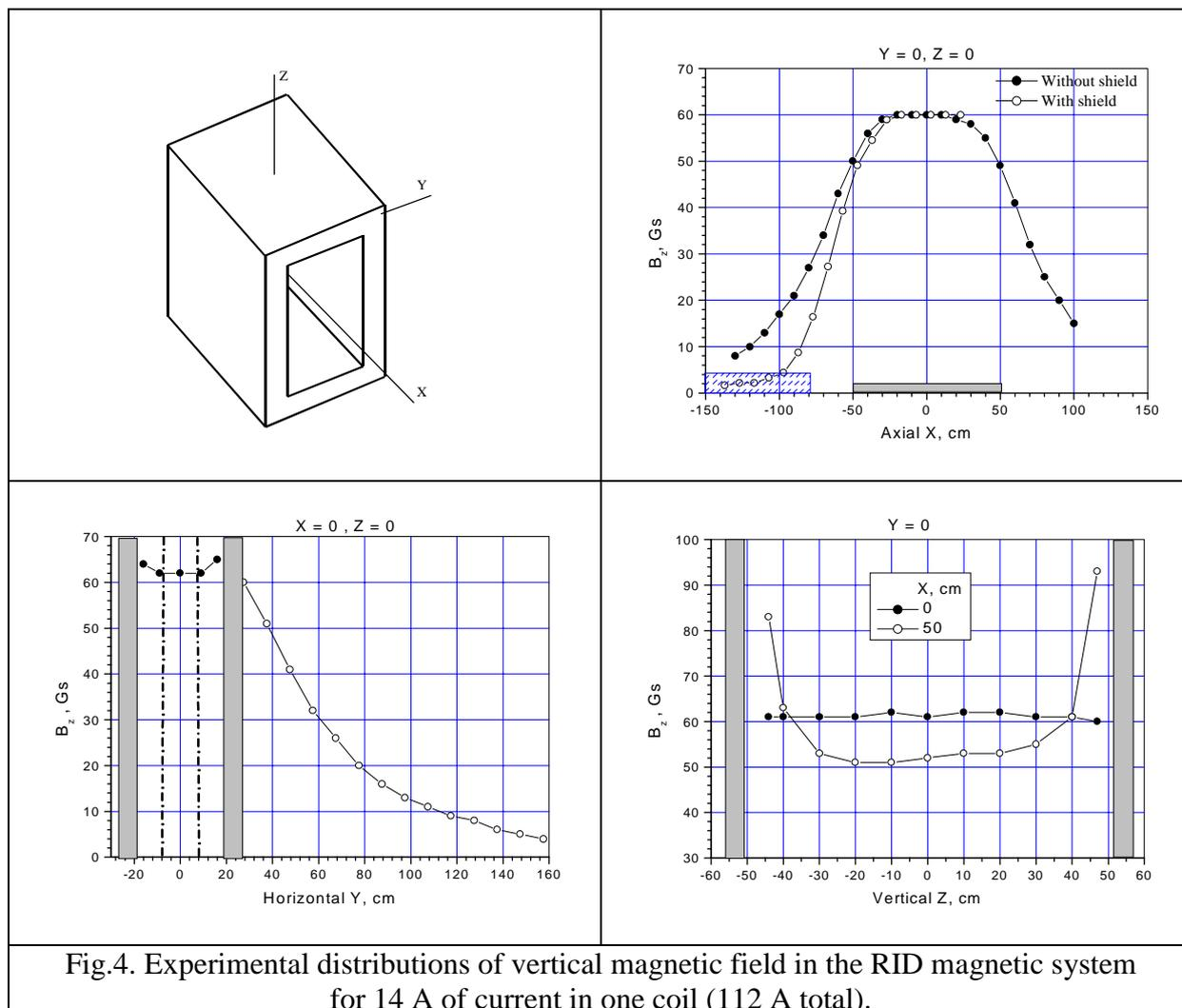
Fig.4. Experimental distributions of vertical magnetic field in the RID magnetic system for 14 A of current in one coil (112 A total).
