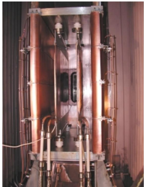
Fig.3. Photos of the RID magnetic system and the RID inside the IREK vacuum vessel (deflecting panel is on the right).
