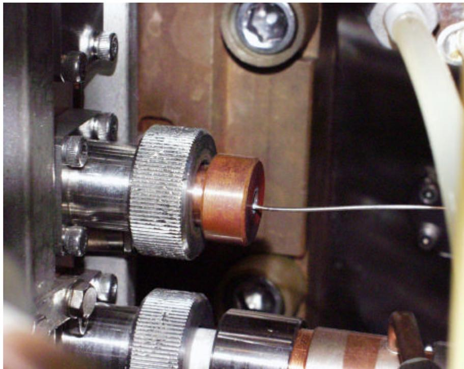
**Figure 4** Typical diagnostic flange on the Kamaboko III ion source. The source body (to the left of the picture) is water cooled copper. The stainless steel adaptor flange is bolted to the source, but this thermally insulates the diagnostic (in this case the copper cylinder with the thermocouple attached) from the source body.
