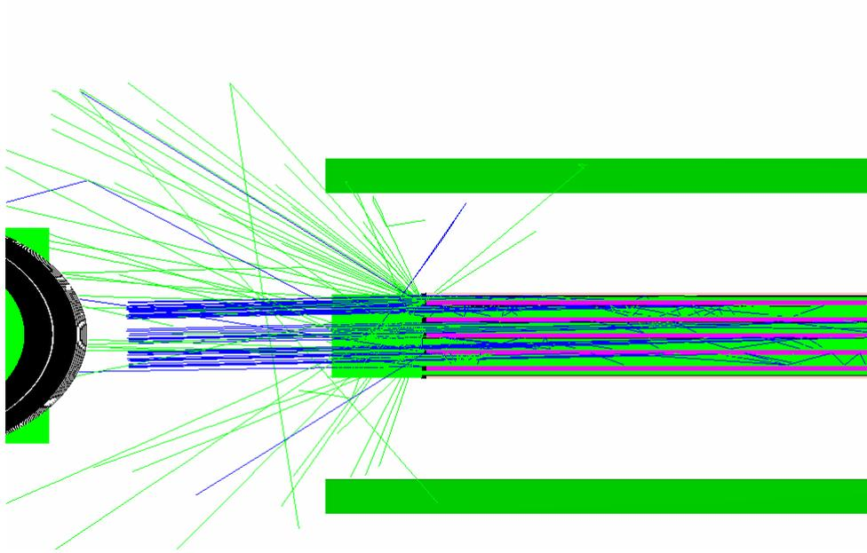
**Figure 11** Calculated tracks of backscattered electrons in the ITER injector.
