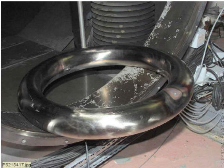
**Figure 10** Photograph of the electrostatic shield damaged by long exposure to the dark current. The arrow indicated the small hole formed by the combination of electron heating and the internal pressure of the ring.
