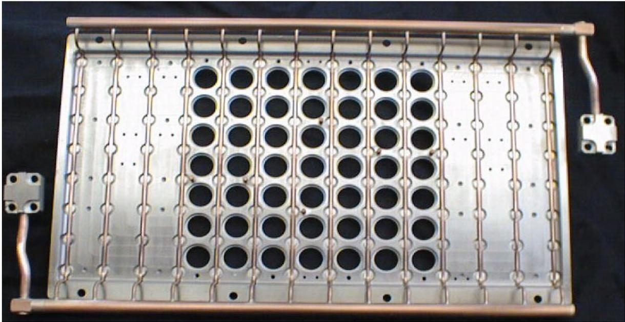
**Figure 3** “Actively cooled” long pulse grid made from molybdenum. The cooling tubes are copper, and the small cylindrical thermal bridges are of stainless steel..
