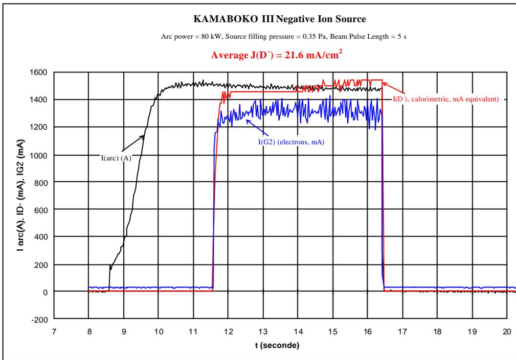
**Figure 1** Kamaboko III ion source: 216 A/m<sup>2</sup> D<sup>-</sup> for a pulse length of 5 s.
