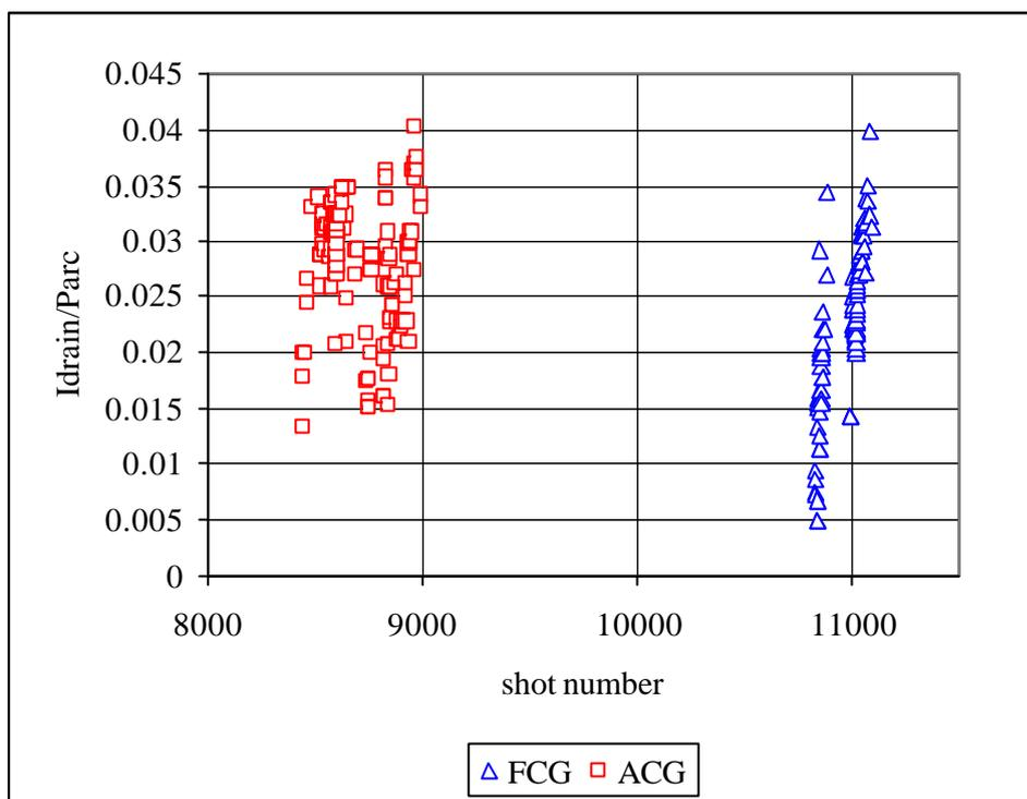
**Figure 7** Comparison of the negative in production efficiency for the Kamaboko III ion source with the two long pulse grids.
