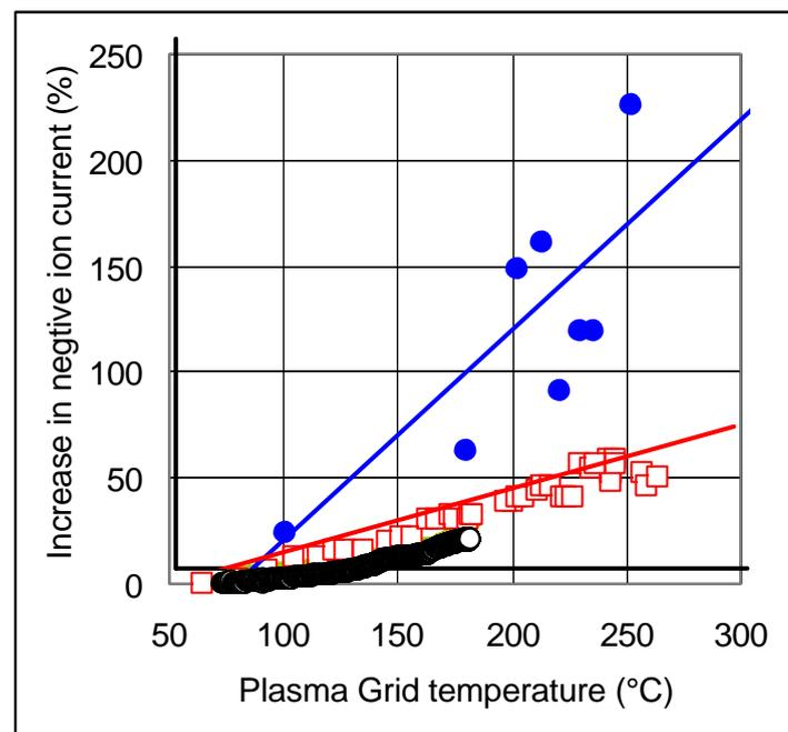
**Figure 6** Increase in negative ion yield from the KAMABOKO III ion source with the plasma grid temperature, arc power  $\approx 50$  kW, source filling pressure  $\approx 0.3$  Pa,  $H_2$  in all cases.
