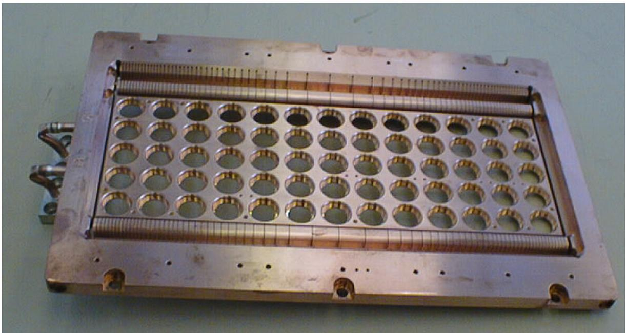
**Figure 2** “Frame cooled” long pulse grid made from copper, chrome zirconium alloy.
