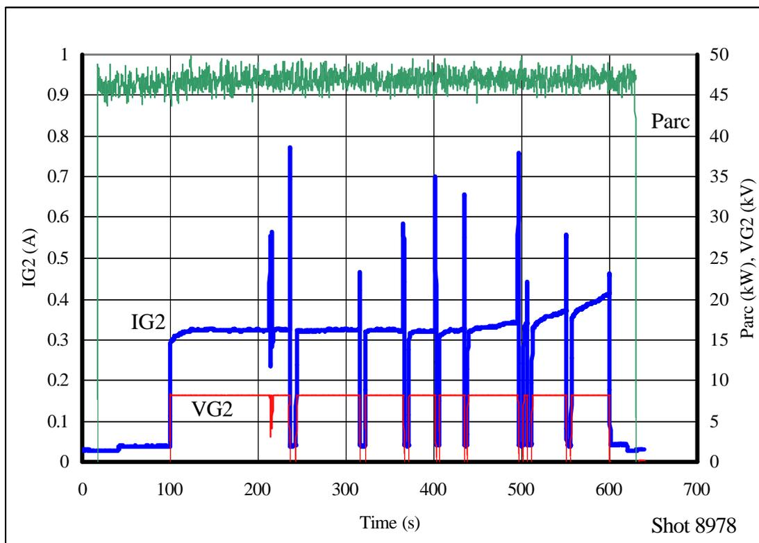
**Figure 8** Example of a pulse of >300 s where the current to the extraction grid (IG2) was seen to run away after  $\approx 450$  s.
