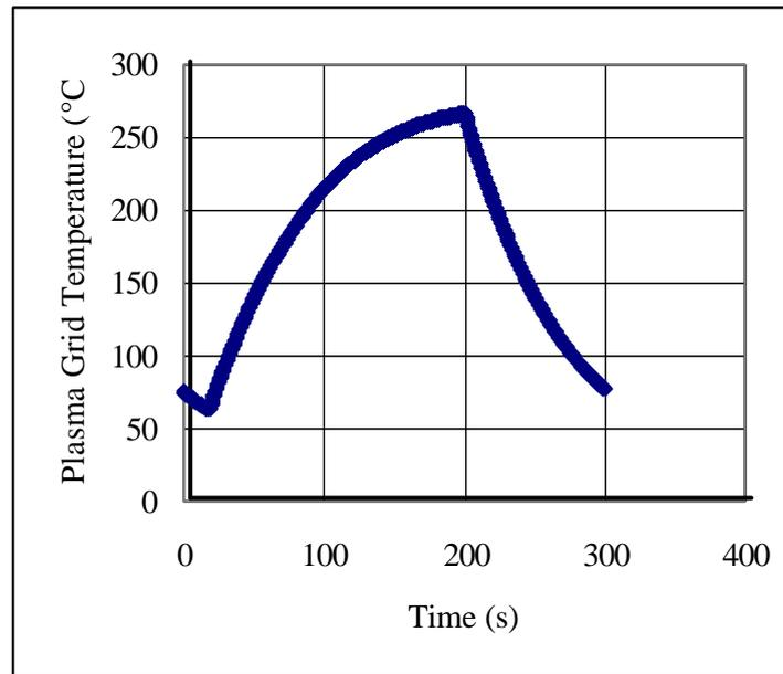
**Figure 5** Temperature of the “frame cooled” long pulse grids during a long pulse with an arc power of  $\approx 45$  kW.
