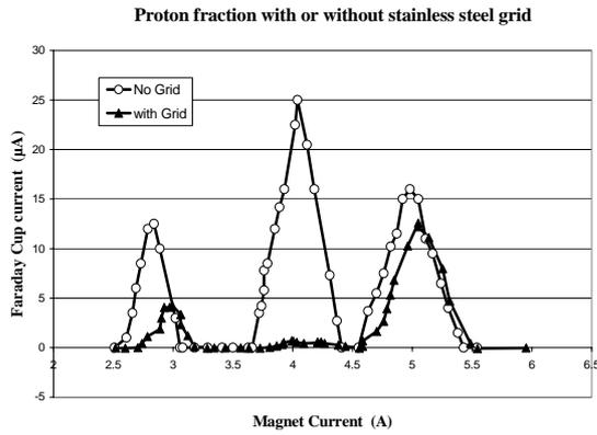
Fig. 1: Positive charge analysis (extracted current vs analyzer magnet) with or without the grid.
