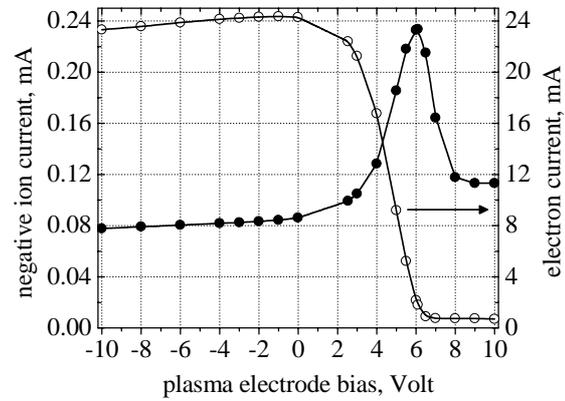
Fig. 4: Variation of the extracted negative ion current and electron current with the plasma electrode bias. Hydrogen pressure 2 mTorr. Applied microwave power 1 kW.
