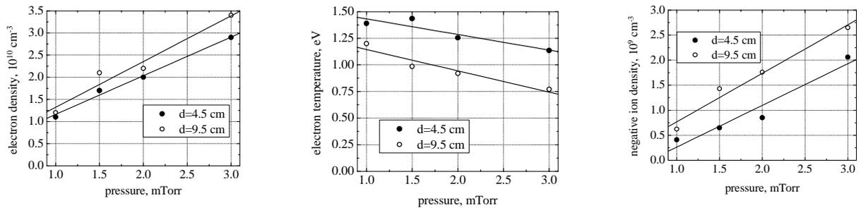
Fig. 2: Dependence of the electron temperature, electron density and negative ion density on hydrogen pressure, for two values of the distance (*d*) between the central minisource and the probe.
