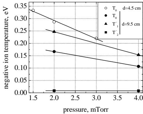
Fig. 3: Dependence on hydrogen pressure of negative ion temperature (average value) at two distances  $d$  from the ECR sources. Two temperature values found for the two  $H^-$  populations for the distance  $d = 9.5$  cm only are also shown. Applied microwave power 1 kW.
