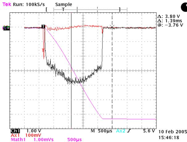
Fig. 5: Extracted pulsed beam (3.8 mA) at low pressure.
