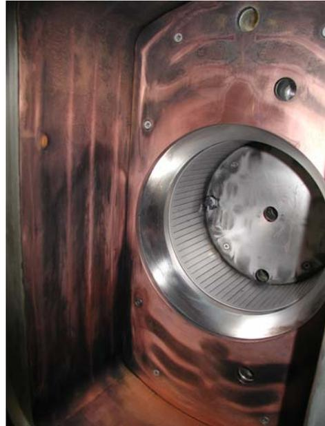
*Fig. 4: View into the cesiated RF source after exposure to air. The cesium oven was located at the top above the dripping marks.*
