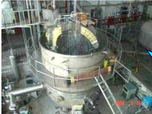
One TF coil inside the cryostat of the test facility
