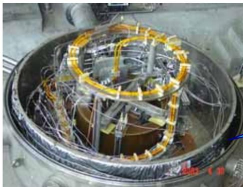
**CS prototype coil inside the cryostat of the test facility**
