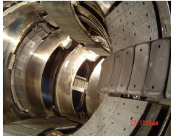
Fig.4 The HT-7 toroidal and poloidal limiters
