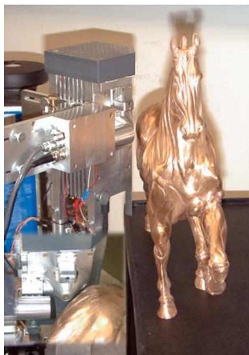
Two groups of samples were analysed: standard reference materials (NBS 1103, NBS 1108, NBS 1115) and selected points on a bronze horse statue. The standards were measured in a sample holder installed on a detachable table. For the measurements of the horse statue the table was removed and the spectrometer was positioned in front of the horse.
