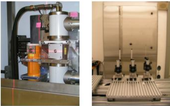
Figure 5: New x-ray calibration and measuring bench for radiotherapy and radiation protection dosimetry
