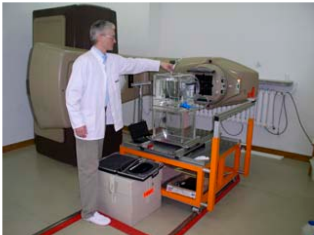
Figure 2. The dedicated Co-60 unit set-up for calibration of radiotherapy dosimeters and for irradiation of TLD powder.
