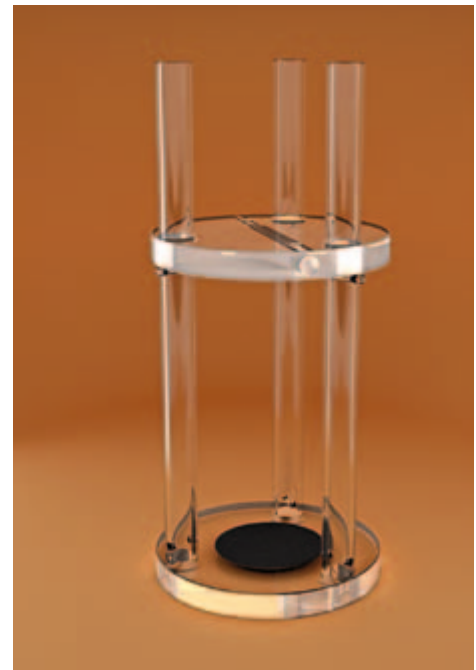
Figure 9. The IAEA TLD holder used for postal dosimetry audits of high energy electron beams.
