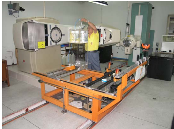
Calibration of an ionization chamber in terms of absorbed dose to water at the SSDL of Bangkok, Division of Radiation & Medical Devices, Department of Medical Sciences (courtesy of S. Smiranoroth)
