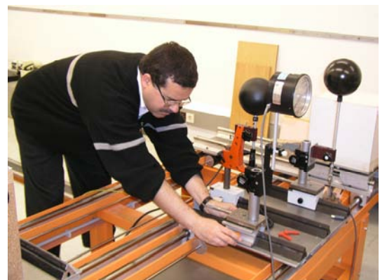
A workshop participant setting up an ionization chamber.
