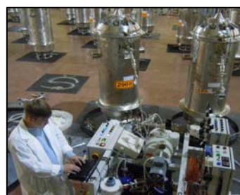
Figure 2: Air tightness test of loaded and closed TUK-19 packages.
