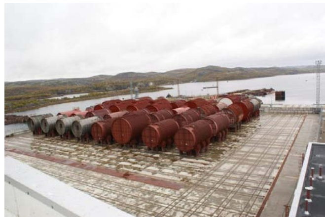
Figure 3: Submarine reactor compartments at the storage facility.
