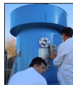
Figure 3: Gamma dose-rate measurement on Skoda
