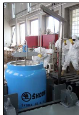
Figure 1: Spent nuclear fuel loading into Skoda VPVR/M
