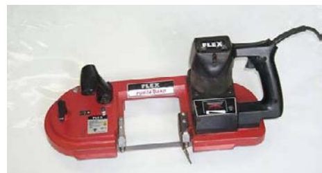
Handheld Mechanical Cutting Equipment (saw) for Small Contaminated Pipes (Courtesy of SCK-CEN, Belgium)
