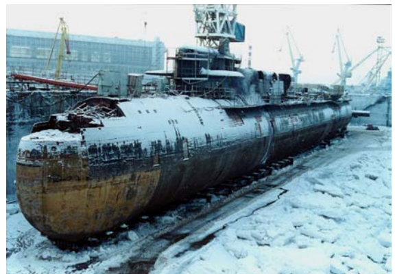
Dismantling a Delta-class submarine at the Zvezdochka shipyard in Severodvinsk, RF (Photo: Courtesy of Zvezdochka shipyard.)
