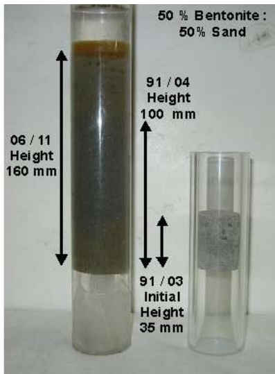
A pellet of swelling clay material made in 1991 (RHS) and in 2006 (LHS) after continuous exposure to water
