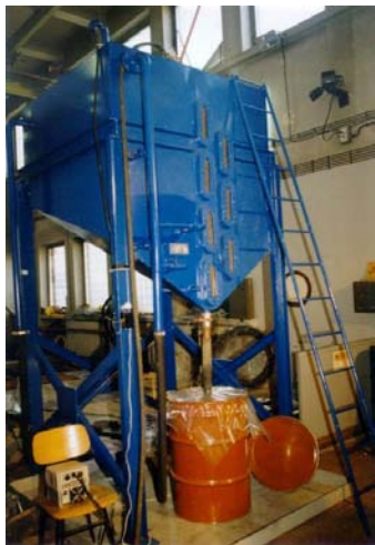
Sludge separation vessel
