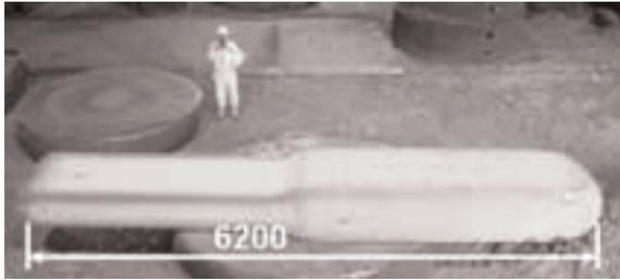
Figure 1. Overview of a ST316LN block at an intermediate stage in the forging process.
