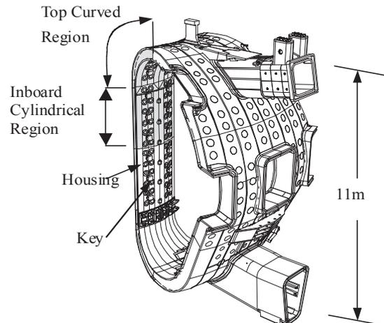
Figure 3. Fabrication of Partial Mock-up of VV.
