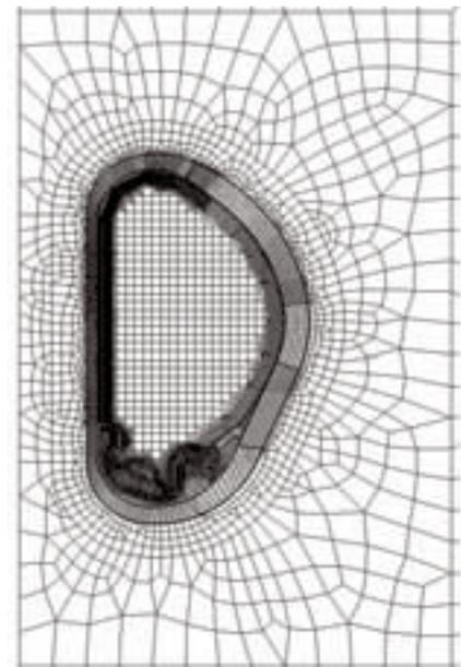
Figure 4. Schematic picture of 3-D solid model of blanket modules, divertor and half sector VV used in electromagnetic analysis of blanket modules.
