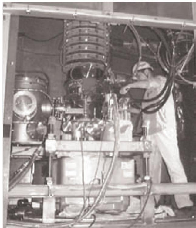
Figure 6. Picture of RF test stand and ITER gyrotron in JAERI.
