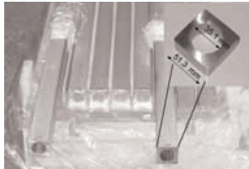
Figure 2. CS circle-in-square jacket section produced in the trial fabrication.
