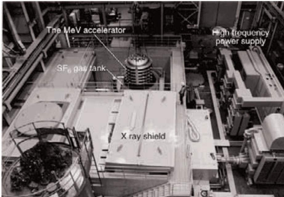
Figure 5. MeV test facility and the vacuum insulated accelerator for 1 MeV, ampere class H<sup>-</sup> ion beam test.
