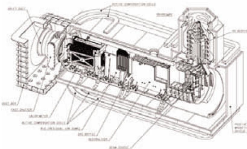
*Scheme of the neutral beam injector for ITER.*
