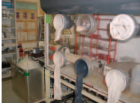
FIG. 18. Uranium/plutonium by K-edge X ray densitometry (HKED).
