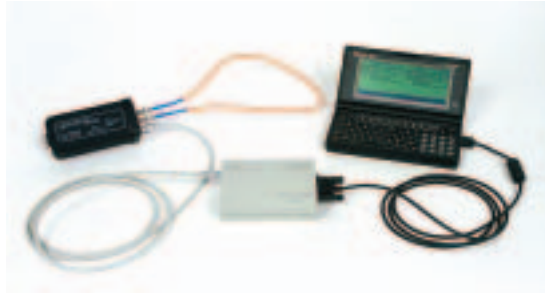
FIG. 34. VACOSS-S Electronic Seal with fibre optic loop, interface box and palmtop computer.
