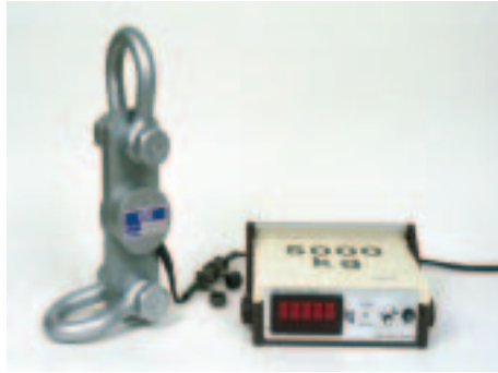
FIG. 13. LCBS: Load Cell Based Weighing System.
