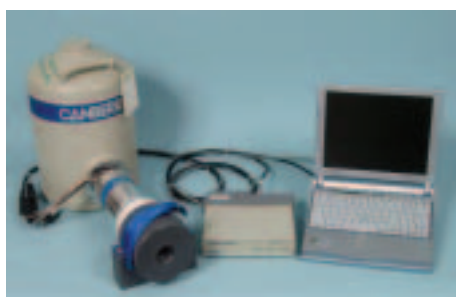
FIG. 5. IMCG: Inspector Multichannel Analyser with HpGe detector.
