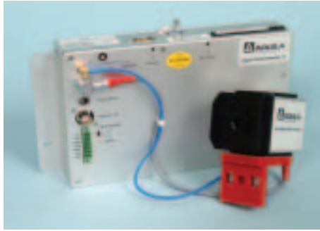
FIG. 22. DCM14 with video CCD camera (CCD: Charge Coupled Device).
