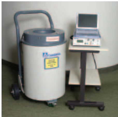
FIG. 8. AWCC: Active Well Coincidence Counter.
