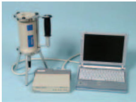
FIG. 3. IMCA shown with an NaI detector and portable computer.
