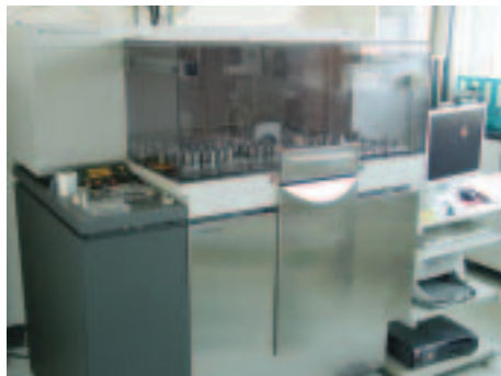
FIG. 19. X ray fluorescence spectrometer.
