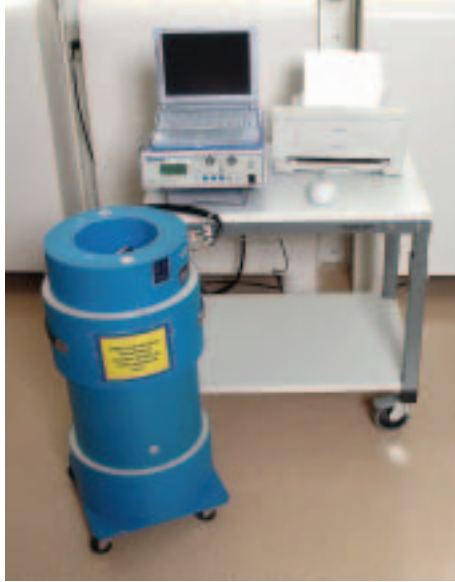
FIG. 6. HLNC: High Level Neutron Coincidence Counter.
