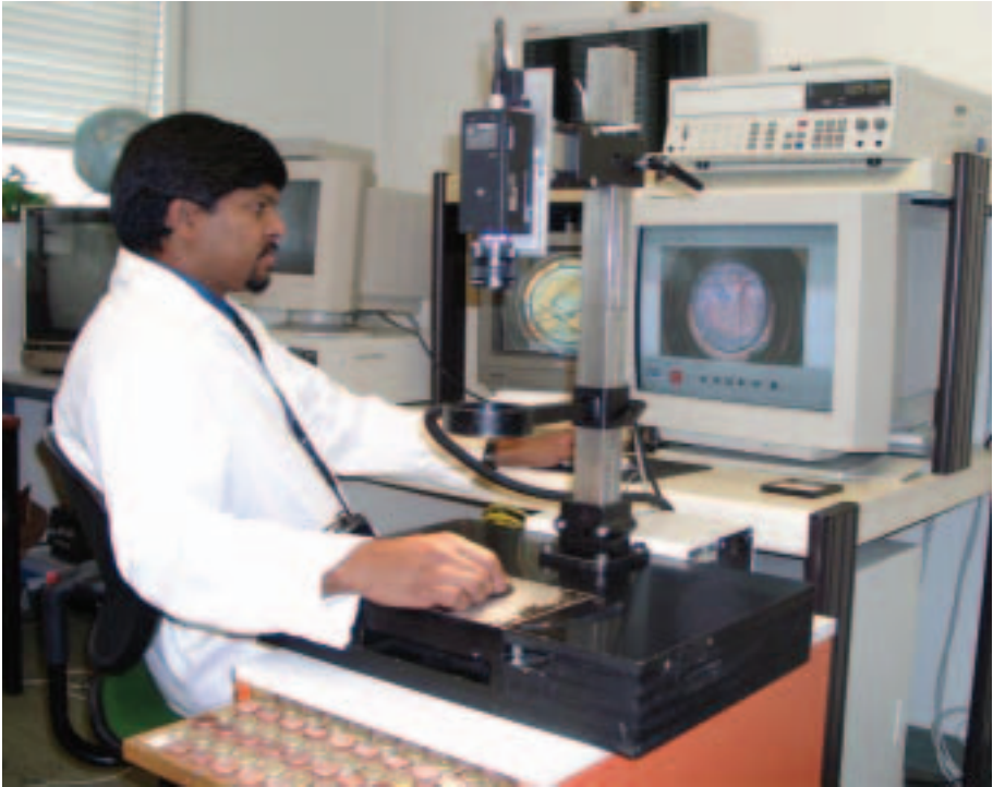
FIG. 32. Comparison of metal cap seal images for seal validation.
