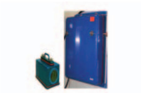
FIG. 24. DSOS: Digital Single Camera Optical Surveillance System.
