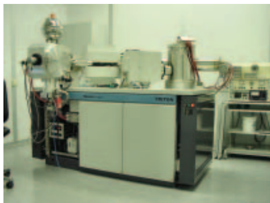
FIG. 44. Mass spectrometer for environmental isotopic analysis.
