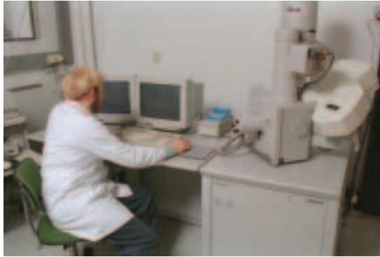
FIG. 45. Scanning electron microscope for particle analysis.
