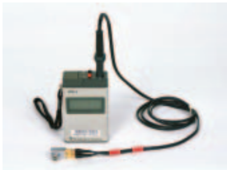
FIG. 14. ULTG: Ultrasonic Thickness Gauge.
