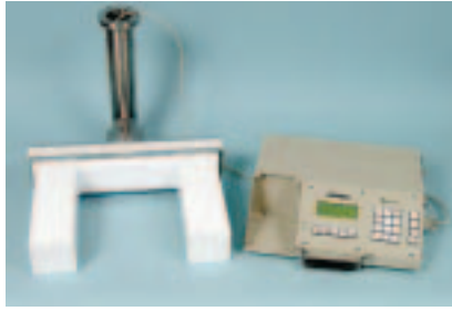
FIG. 9. FDET: Fork Detector Irradiated Fuel Measuring System (detector head, GRAND electronics unit and portable computer).
