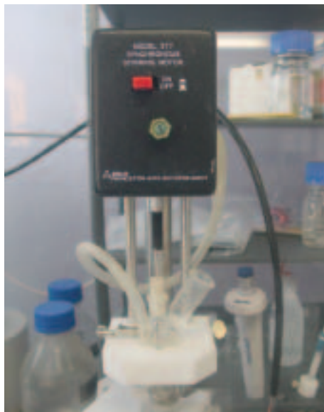
FIG. 17. Coulometry cell for determination of Pu concentration.
