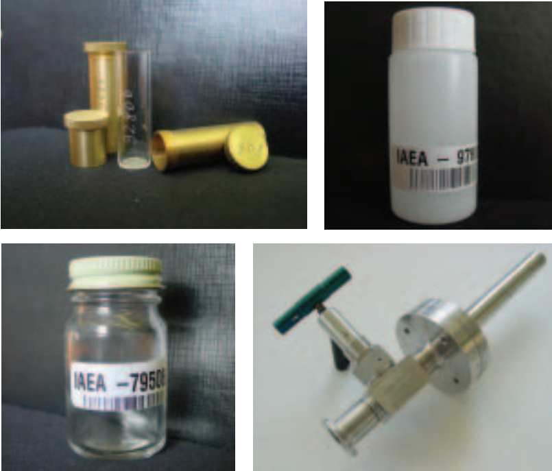
FIG. 15. Sample bottles used for IAEA verification samples. Top left: vials for Pu, MOX or high enriched U powder. Top right: hard polyethylene bottle for hard or solid materials. Bottom left: glass bottle for depleted, natural or low enriched U powder. Bottom right: UF_6 container.
