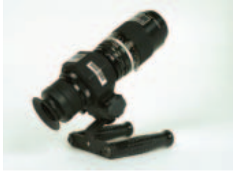
FIG. 12. ICVD: Cerenkov Viewing Device.
