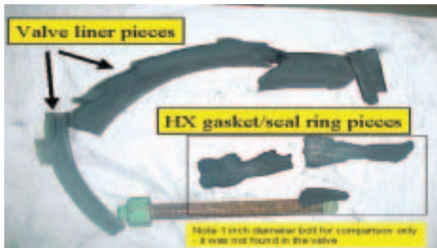
Debris found in the valve (A 1" diameter bolt is placed beside the debris for comparison.)
