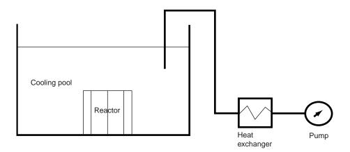
The event to be rated is one where the pipework downstream of the pump failed and coolant was pumped out to the bottom of the suction pipe. The pump then failed owing to cavitation.
