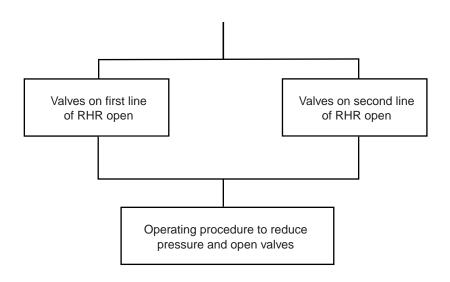
The reliability of the safety provisions is limited by the need for operator action. Given the complexity of the operation and the limited time available, it is considered that there is only one effective safety layer, i.e. an operating procedure requiring pressure reduction and reopening of the isolation valve. Again, therefore, level 3 is considered appropriate.
