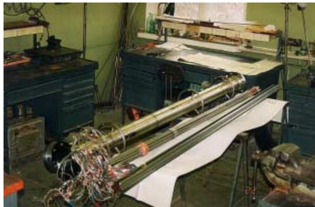
FIG. 4: Test Channel with the 19 rod bundle simulator.
