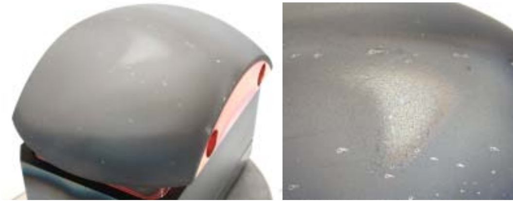
Fig. 9. The surface of a test limiter (made of copper coated with 170\ \mu\text{m}\ \text{B}_4\text{C} ) after 80 exposures in TEXTOR near the last-close flux surface. The melting zone is clearly seen especially in the magnification at the right hand side where also a number of craters are visible possibly caused by electrical arcs.
