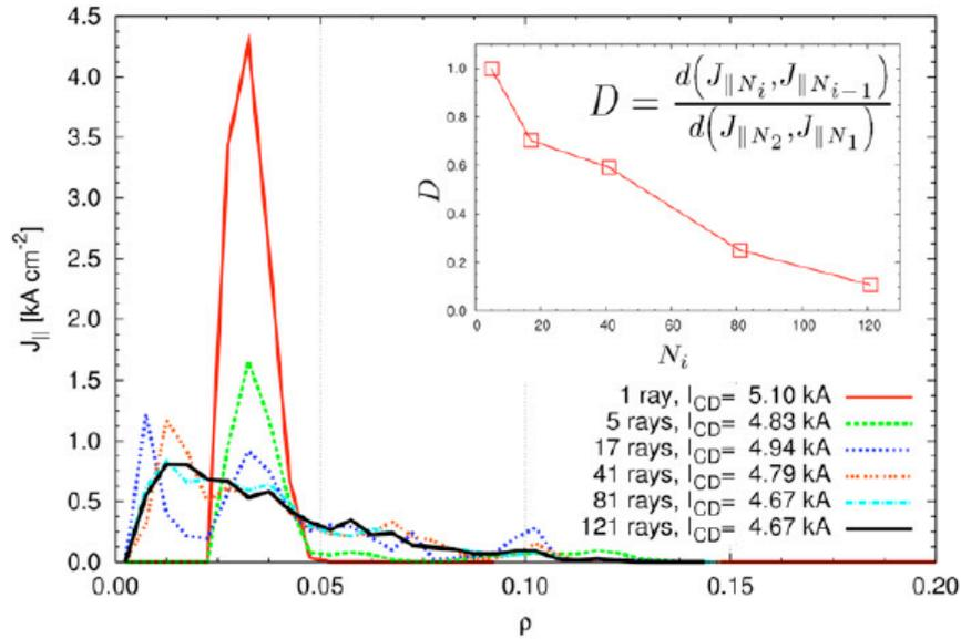
**Figure 4.** Electron Bernstein current driven profiles for several number of launched rays. It is seen that a number as high as 121 rays is enough to get reasonable level of convergency and gives an accurate enough value for the current.
