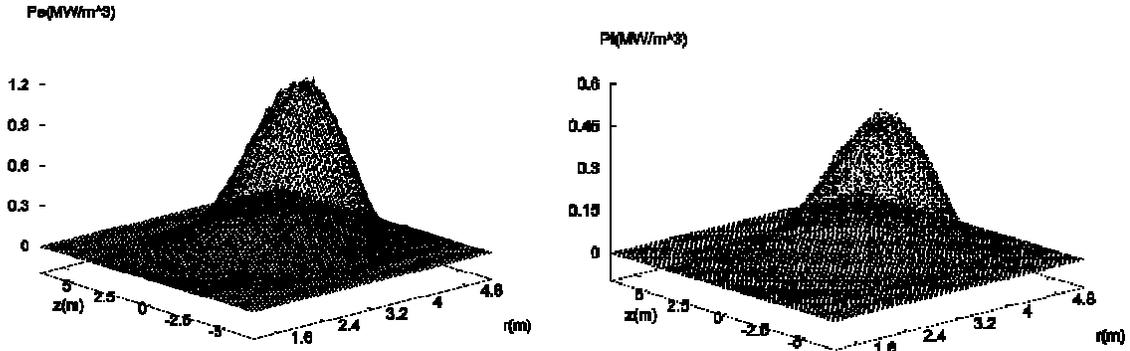
Fig. 4. Power deposited in electrons and ions for an S2 equilibrium.
