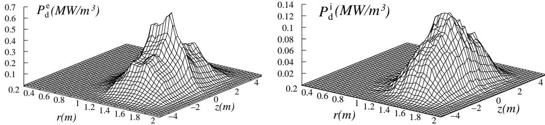
Fig. 1. Power deposited in electrons and ions
