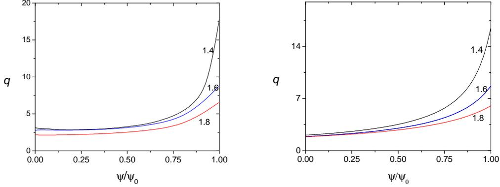
Fig. 3.  $q$  profiles, as a function of poloidal flux, for different aspect ratios. Left E1-E3, right S1-S3
