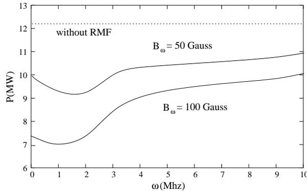
Fig. 2. Power deposited as a function of the RMF frequency;  $\delta=0.1 r_s$
