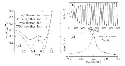
**FIG. 2**. Antenna excitation of n = 4, m = 7 RSAE with kinetic thermal ions using GTC. (a) m = 7 Alfven continua and eigen-frequencies obtained from GTC simulations, with and without thermal ions. (b) Time history of electrostatic potential  $\delta\phi$  for antenna frequency  $\omega_{ant} = 0.195 v_A/R_0$  showing saturation of the mode. (c) Saturated  $\delta\phi$  amplitude versus antenna frequency and best fit to estimate the RSAE damping rate.
