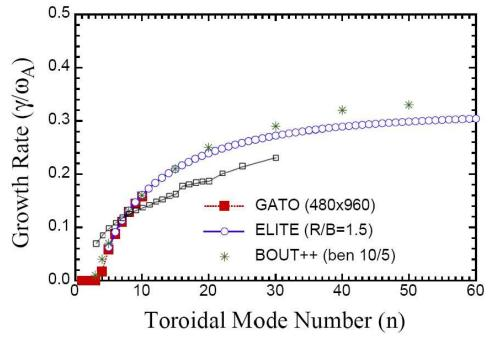
Fig. 8: GTC simulation of ideal ballooning mode: linear growth rate as a function of n, compared to the results from several fluid codes in Ref. [25].
