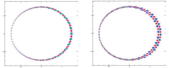
**Fig. 6**: GTC simulation of ideal ballooning mode: poloidal contour plot of electrostatic potential (left) and vector potential (right).
