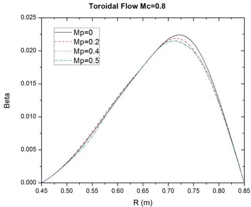
Figure 8: Effect of poloidal flow on beta profile, at sonic speed
