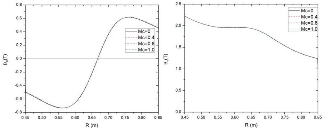
Figure 2: Poloidal B and Toroidal B with with varying toroidal Mach speed
