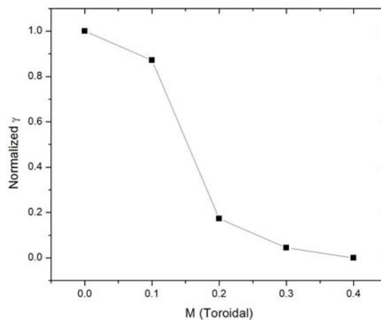
Figure 10: Instability growth rate as a function Toroidal flow
