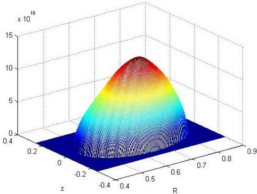
Figure 7: 3D density plot for equilibrium arbitrary flow (where density is in  $\#/m^3$ )
