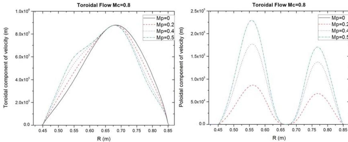
Figure 6: Toroidal velocity (left) and poloidal velocity (right) variation with poloidal flow at constant toroidal flow ( $M_c=0.8$ ).
