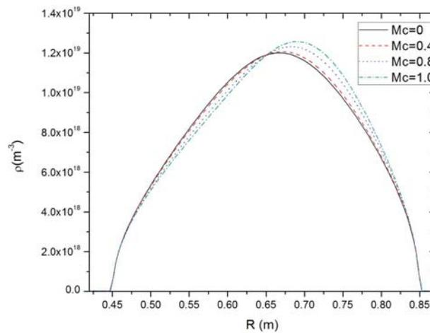
Figure 1: Density variation with varying toroidal flow
