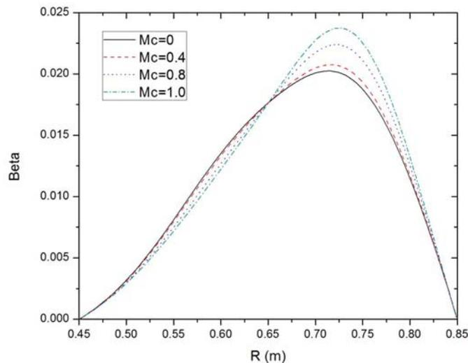
Figure 4: Beta variation with purely toroidal flow.
