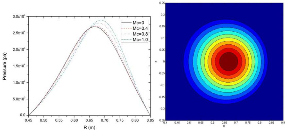
Figure 3: Variation of Plasma pressure (left) and (right) shows the shifted contours of poloidal flux function corresponding to sonic toroidal flow ( $M_c=1$ )
