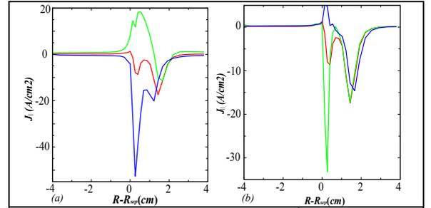
FIG. 5. The profiles of  $J_{\parallel}$  (A/cm<sup>2</sup>) on the OSP for: (a) reference case (red), ISP biased to +50 V (green), OSP biased to +50 V (blue); (b) reference case ( $A_n=98\%$ , red), enhanced OSP pumping ( $A_n=90\%$ , green), no OSP pumping ( $A_n=100\%$ , blue).
