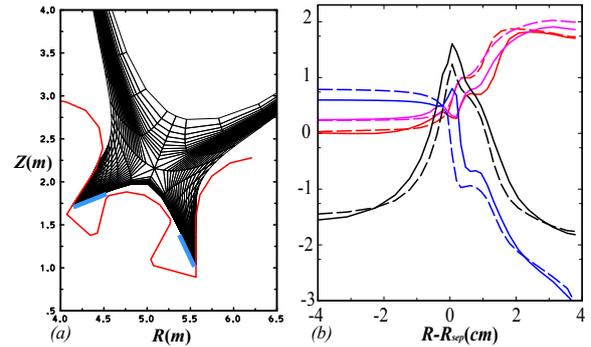
FIG. 4. (a) The ITER mesh (black), approximate geometry of the divertor baffle (red), and pump/injector regions (blue). (b) The plasma conditions on the target plate in the reference case vs. distance on the outer midplane:  $\log_{10}$  scale for  $T_e$  (eV, red),  $T_i$  (eV, magenta),  $n_i$  ( $10^{20} \text{ m}^{-3}$ , black), and  $n_n$  ( $10^{20} \text{ m}^{-3}$ , blue).
