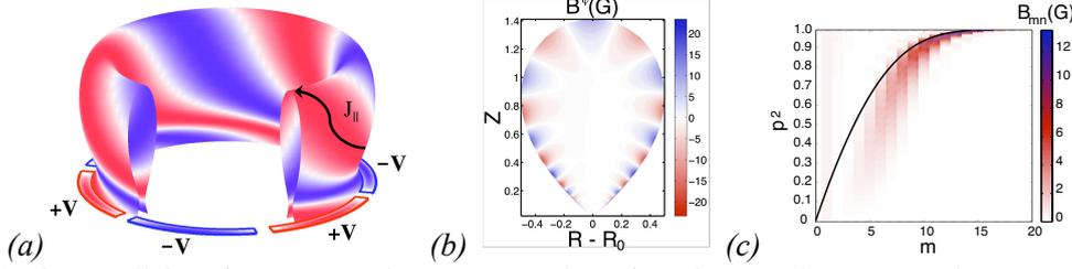
FIG 2. (a) The parallel surface current density  $K_{\parallel}$  resulting from biasing the target with 6 segments. (b) The magnetic perturbation field in the two-wire model of a plasma equilibrium produced by  $K_{\parallel}=10$  kA/m at a higher mode number. (c) At the edge ( $p^2=1$ ), the poloidal spectrum is peaked near  $m=qn$  (black line).
