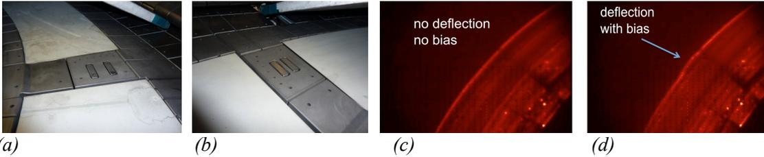
FIG 3. Two pairs of biasable electrodes were recently installed on the NSTX outer divertor plates: (a) toroidally oriented pair and (b) radially oriented pair. The white surfaces are the newly installed liquid lithium divertor plates. Top-down views of the toroidal pair in (a) as viewed in LiI light: (c) no bias and (d)  $\pm 90$  V bias. Turbulent filamentary structures are observed to bend around the outer positively biased electrode as they pass by.
