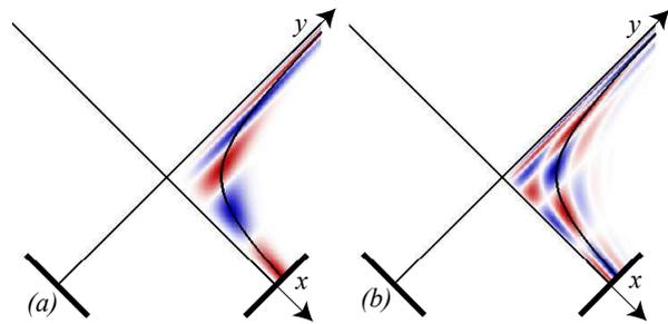
FIG. 1. Field-aligned structure of the non-axisymmetric parallel current and electrostatic potential in the X-point region generated by perturbations to the divertor plasma. On the target plate, the perturbation varies (a) in the toroidal direction only and (b) in both the radial and the toroidal directions.
