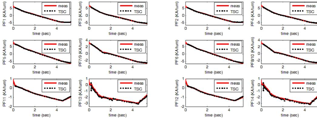
FIG. 2. Shot 16028 PF current (KA/turn) versus time (sec). (left) PF coils with the odd number, (right) PF coils with even number. PF7 and PF9, PF8 and PF10 connected together, respectively. In the figure, the measurements are shown by red line and the TSC simulated data by black dot line.
