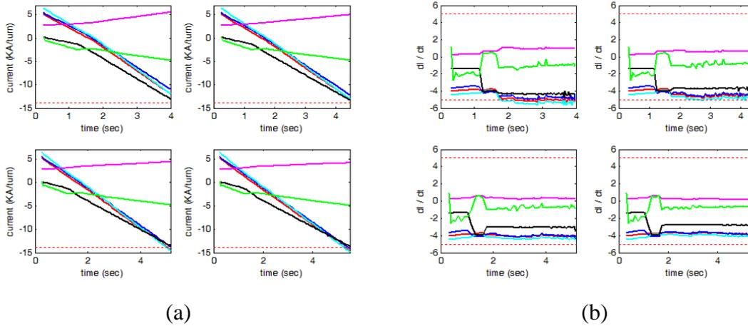
FIG. 9. (a) PF current trajectories (PF1-red, PF3-blue, PF5-cyan, PF7/9-magenta, PF11-black, PF13-green) versus time for ramp-up time 4.0 sec (top left), 4.46 sec (top right), 5.14 sec (bottom left), and 5.50 sec (bottom right). 95% PF current limitation is signed by red dot. (b) PF currents change rate trajectories (same setting to Fig. 9(a)) versus time for the fourth condition. The maximum PF change rate is signed by red dot.
