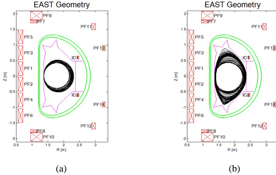
FIG. 1. The evolution of plasma boundary (black line) of (a) shot 16028 (limiter), and (b) shot 17126 (divertor) plot in the EAST geometry. The green lines sign EAST double layer vacuum vessel, and the magenta line is the EAST limiter components.
