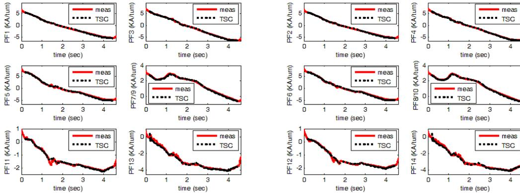
FIG. 6. Shot 17127 PF current (KA/turn) versus time (sec). (left) PF coils with the odd number, (right) PF coils with even number. PF7 and PF9, PF8 and PF10 connected together, respectively. In the figure, the measurements are shown by line and the TSC predictive data by dot line.
