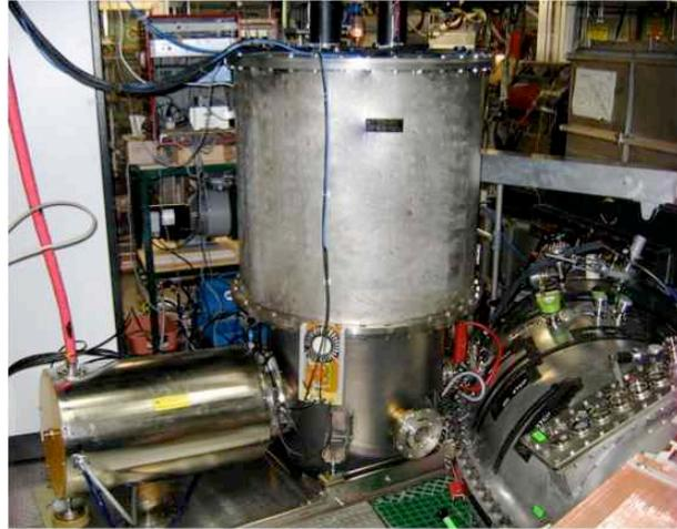
FIG. 4. Compact neutral beam injector.
