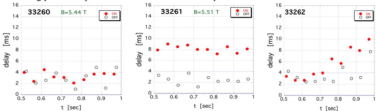
**Fig. 4.1:** Delay between sawtooth crash and ECRH switch on (red filled) and switch off (black empty).  $P_{ECRH} = 0.77 MW$ , modulated: 10 ms on and 40 ms off
