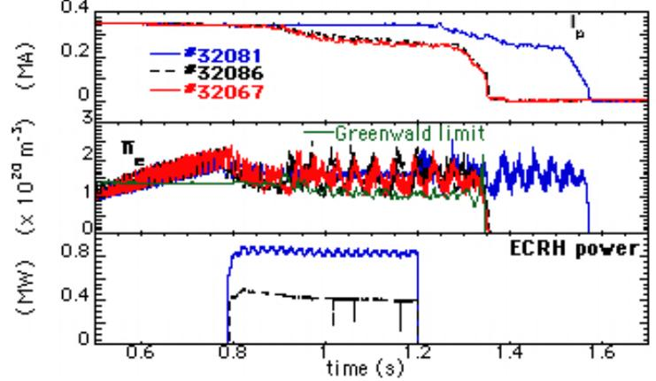
**FIG. 4.2:** Time traces from top of  $I_p$ ,  $\bar{n}_e$  and  $P_{\text{ECRH}}$  in the reference density limit disruption (#32067) and in two discharges with off-axis ECRH (#32081,  $P_{\text{ECRH}} \sim 0.8$  MW; #32086,  $P_{\text{ECRH}} \sim 0.4$  MW)
