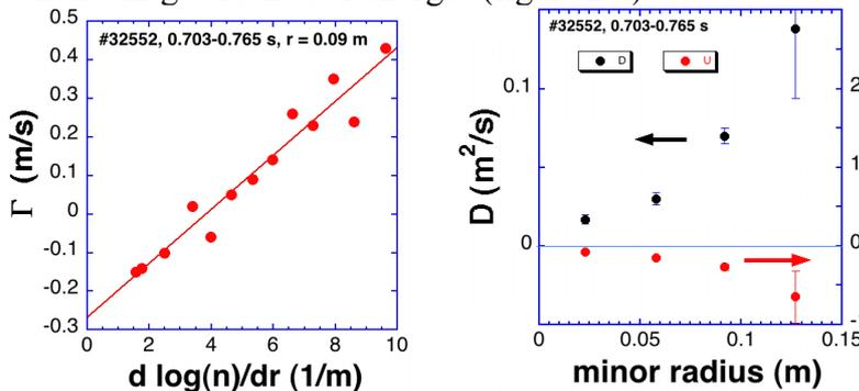
**Fig. 2.5:** Experimental particle flux at  $r = 9\text{cm}$  in the post pellet phase derived from density profiles evolution (left). Diffusion coefficient and pinch velocity versus minor radius (right)
