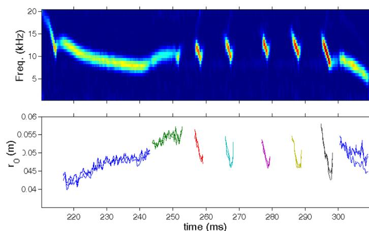
**Fig. 5.1:** Spectrogram of the electron temperature fluctuations (top) and radial position (bottom) of the induced  $T_e$  fluctuations due to e-fishbones in FTU #20865
