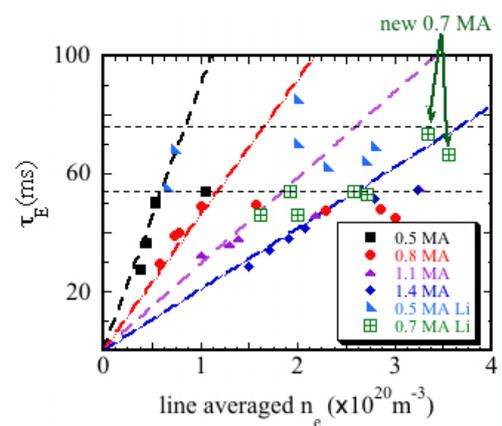
**Fig. 2.1:** Energy confinement time vs line averaged density in ohmic FTU "lithized" discharges.
