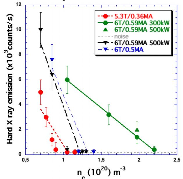
**Fig. 3.1:** LH accelerated fast electrons hard X-ray vs plasma density. Unmodified edge (dashed lines) and high  $T_e$  edge with lithized wall (full line) regimes.
