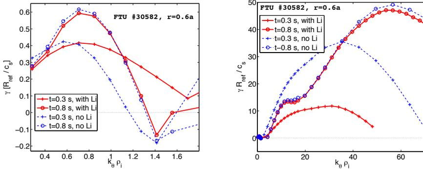
**Fig. 2.2:** Growth rates of ITG (left) and both ITG plus ETG modes (right) for two time slices  $t = 0.3$ s and  $t = 0.8$ s at  $r = 0.6a$  for FTU shot #30582. Results with same parameters but without Lithium (dashed). Here  $\rho_i = \rho_D$
