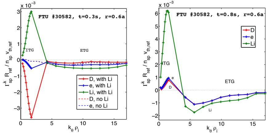
**Fig. 2.3:** Spectrum of three species particle flux (red: D, blue: e<sup>-</sup>, green: Li) driven by ExB convection of ITG and ETG modes. Left  $t = 0.3$ s, Right  $t = 0.8$ s. Results with the same parameters but without Li (dashed)
