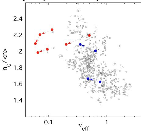
**FIG. 4.3:** Density peaking vs  $\nu_{\text{eff}}$  in OH FTU discharges ( $B_T = 6\text{T}$ ,  $I_p = 0.55\text{MA}$ ) (open gray symbols), EC heated discharges (red and blue dots). Arrows point from OH to RF heated phase
